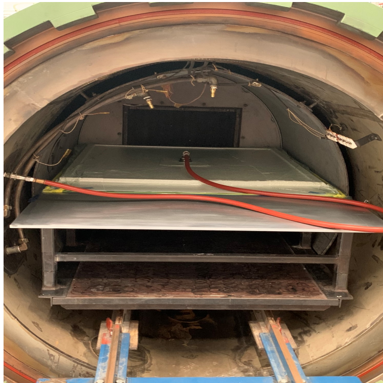
Figure 5.8: Panel ready for curing in the autoclave
