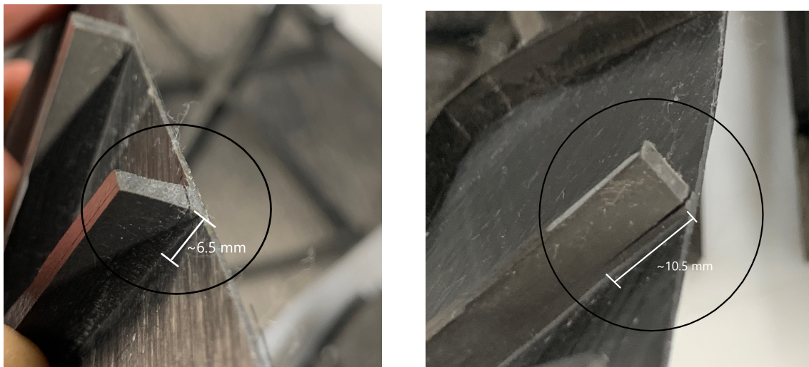
Figure 6.2: Helical ribs delamination
