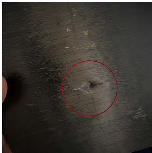
Figure 6.8: Specimen P2-C8-BV, 36J
