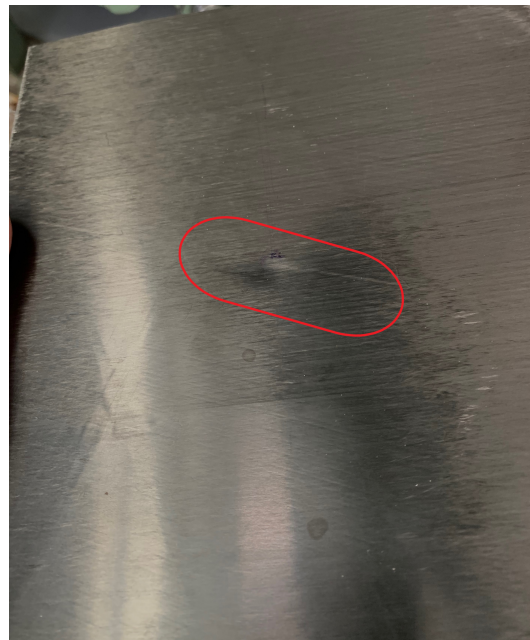
Figure 6.6: BVID, specimen P1-C5-VD, 27J
