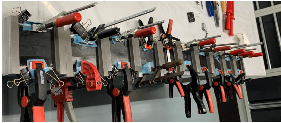
Figure 5.15: Clamped edges support during curing
