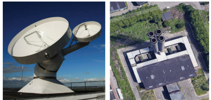
Fig. 14. PARSAX (left) and measured industrial chimney at approximately 1185 m from the radar sensor (right).
