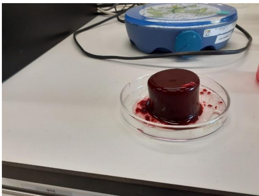
Figure S18. Gelation of crude amic acid reaction mixtures. The hydrogels contain 0.5-1% w/w amic acid, DBU-Cl salts, excess amine and ~10% DMF.
