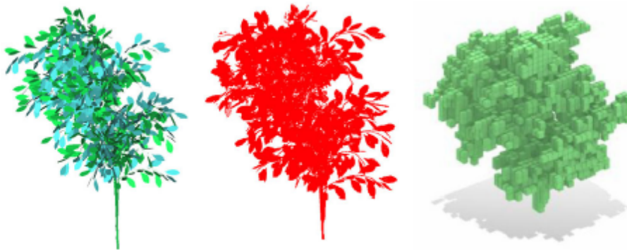
Figure 4.2: Triangle mesh, point cloud and voxel representations [1]
