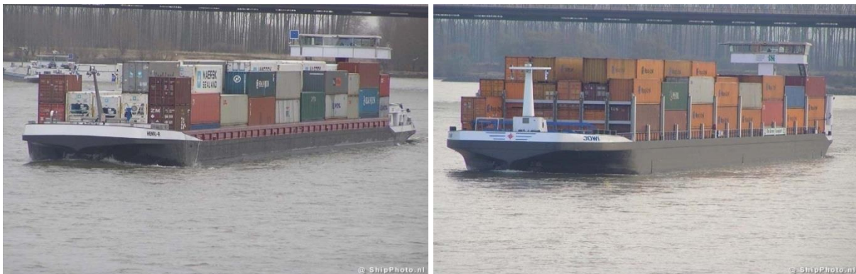
Figure 2-16: Class VI Container barges with 5 (Left) and 6 (Right) Containers Wide
