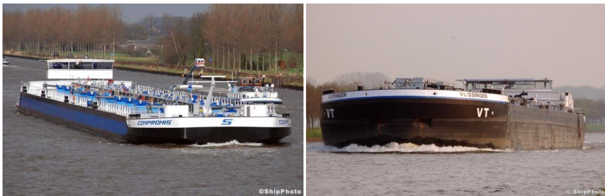
Figure 2-17: Class VI Oil Product Tankers of 15 meter (Left) and 22 meter wide (Right)
