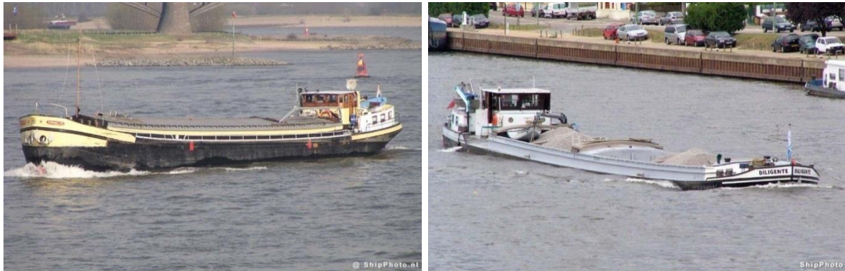
Figure 2-10: Class I Barge (Left) and Class II Barge (Right)
