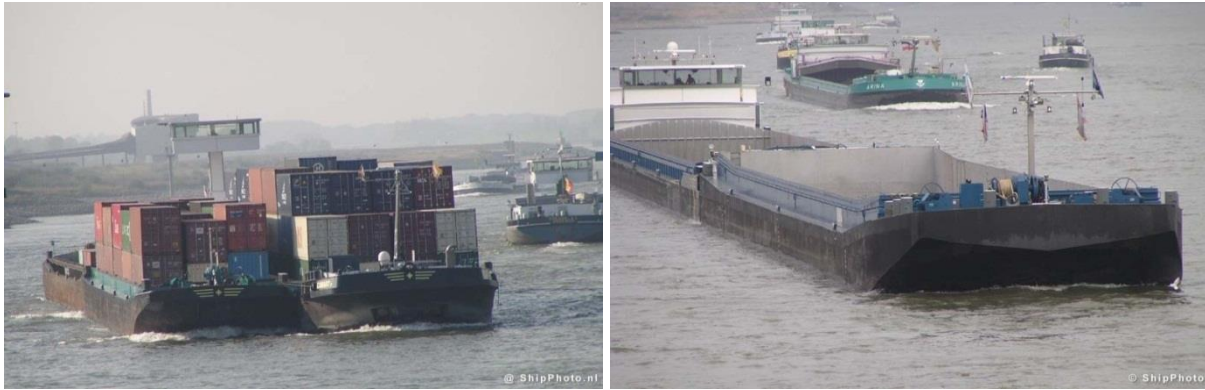
Figure 2-15: Class V coupled unit with dumb barge aside (Left) and in front (Right)
