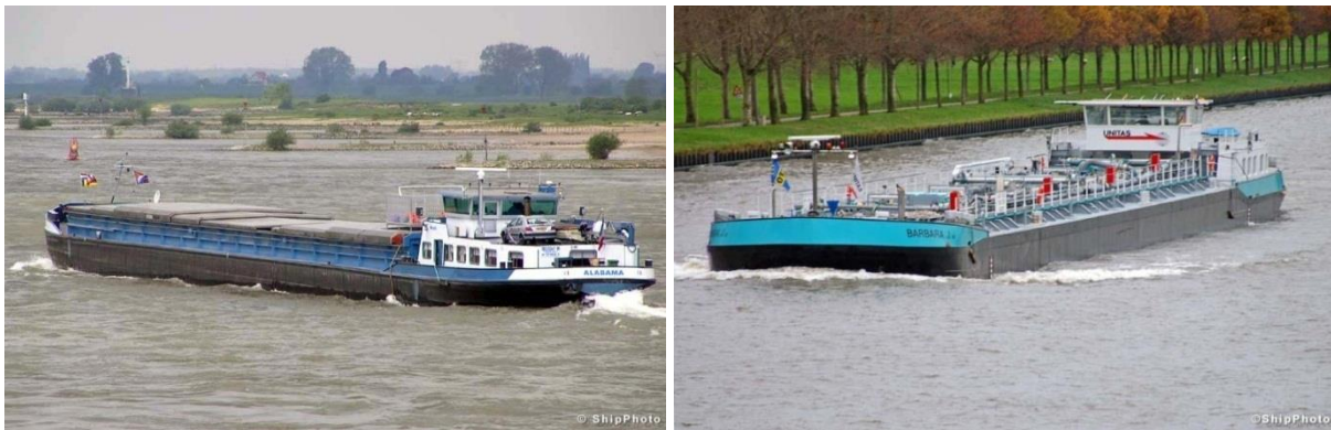
Figure 2-12: Class IV Dry Bulk Barge (Left) and Tanker (Right)
