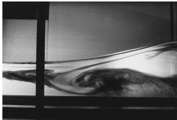
Figure 2.7: Dye pattern depicting vortex structure beneath the wave trough [ Li and Dalrymple, 1998 ]. The wave propagates to the left side in this figure.
