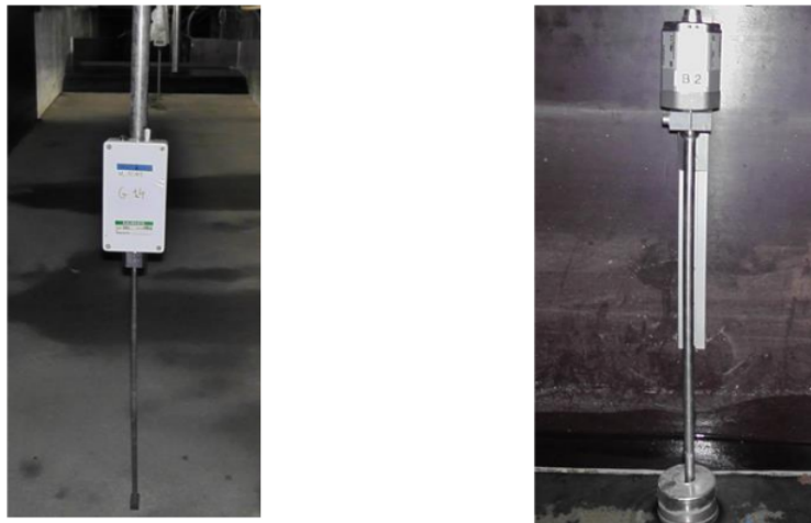
Figure 4.8: Wave gauge (left image) and micro-pulse transducer (right) used to measure the water level in the overtopping box.
