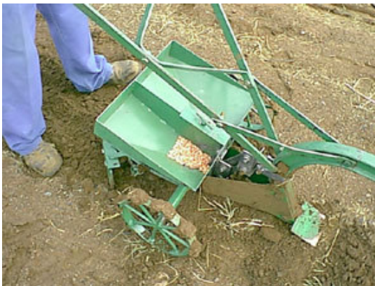
Figure 4.2: Ripper with direct seeding tray
