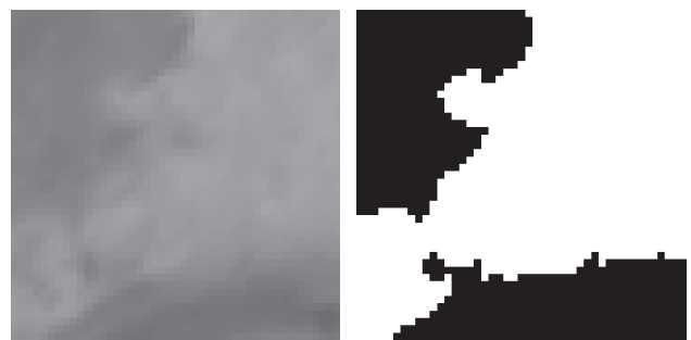
FIGURE 5: NDVI map on which a threshold is used to obtain the tiles that contain vegetation. Threshold is set at 0.08.
