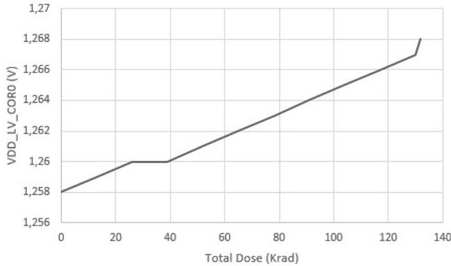
Fig. 4.  $^{90}\text{Sr}$  TEST: Behavior of the  $V_{\text{core}}$  voltage
