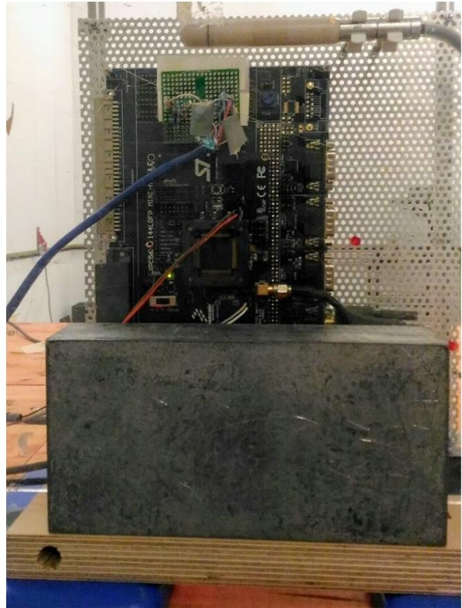
Fig. 5. Test Setup for  $^{60}\text{Co}$  test
