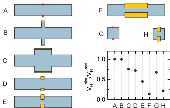
**Fig. 3** Simulation of the Hall voltage  $V_H^{\text{sim}}$  for different device and contact geometries: high aspect ratio nanofins with 'ideal' contactless probes (A), a classic Hall bar (B), wide recessed Hall probes (C), device with short metal probes (D), long metal probes (E), wide metal probes (F), low aspect-ratio nanofin with 'ideal' contactless probes (G), and invasive contacts (H).  $V_H^{\text{sim}}$  is normalized to the 'real' Hall voltage  $V_H^{\text{real}}$ .
