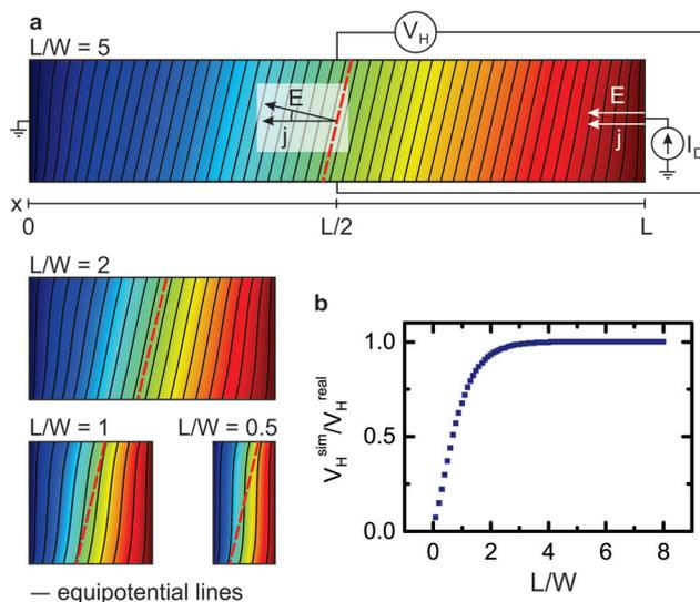
**Fig. 4** (a) Equipotential lines for four different  $L/W$  aspect ratio samples at magnetic field  $B = 0.75$  T. The red dashed line indicates an equipotential line corresponding to the Hall angle of  $V_H^{\text{real}}$ . (b) Transverse voltage drop  $V_H^{\text{sim}}$  at the sample's centre normalized to  $V_H^{\text{real}}$  vs. sample aspect ratio  $L/W$ .
