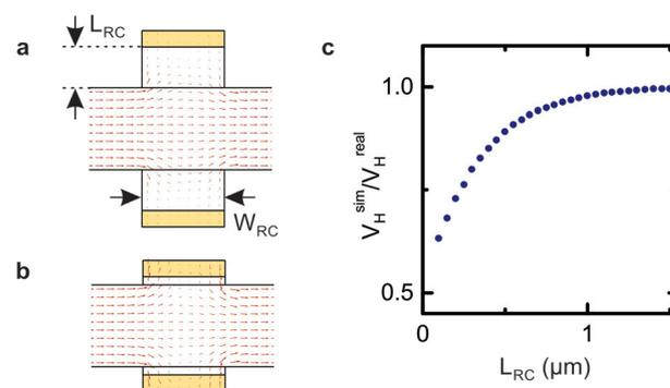
**Fig. 6** Simulated current density for a  $5 \mu\text{m} \times 1 \mu\text{m}$  nanofin with 1  $\mu\text{m}$  wide and (a) 0.5  $\mu\text{m}$  and (b) 0.1  $\mu\text{m}$  long recessed contacts. (c)  $V_H^{sim}/V_H^{real}$  vs. recessed contact length  $L_{RC}$  for this device geometry.
