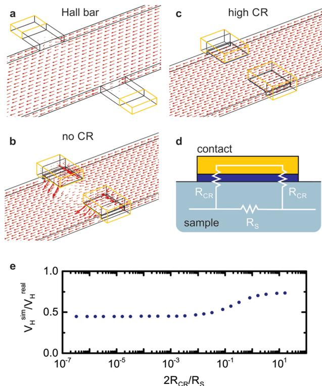
**Fig. 5** Simulation of current density (red arrows) in (a) a classic Hall bar, (b) sample with 'invasive' low contact resistance metal probes, and (c) sample with high contact resistance metal probes. (d) Schematic of the two competing current paths through the sample and the contact in the probed segment.  $R_{CR}$  is the contact resistance and  $R_S$  is the resistance of the segment below the contact. (e)  $V_H^{sim}/V_H^{real}$  for different contact  $2R_{CR}/R_S$  ratios.
