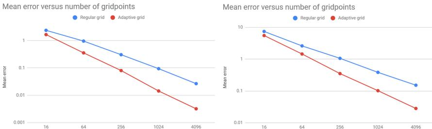
Figure 6.15: The mean error comparison between automatic non-uniform and uniform parameterization at different parameterization resolutions for both operators
