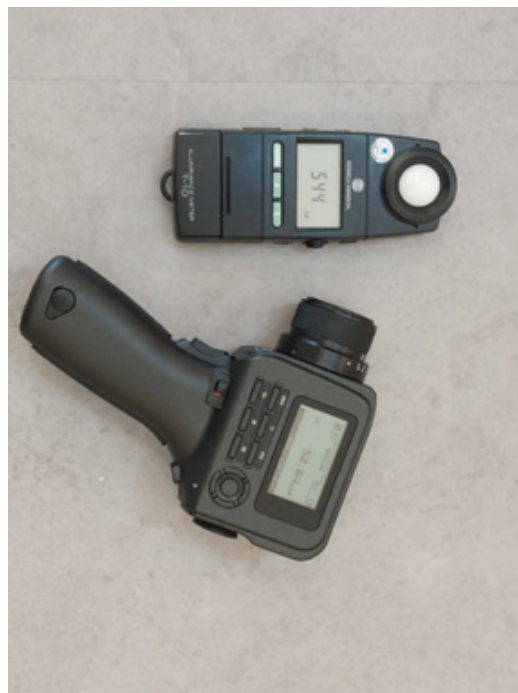
Figures 15 and 16: The spot measurement set up and measuring the reflectance
