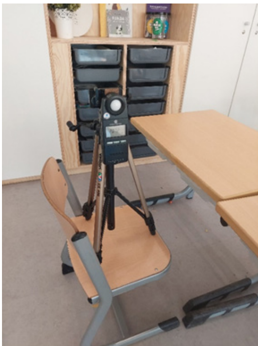
Figures 15 and 16: The spot measurement set up and measuring the reflectance
