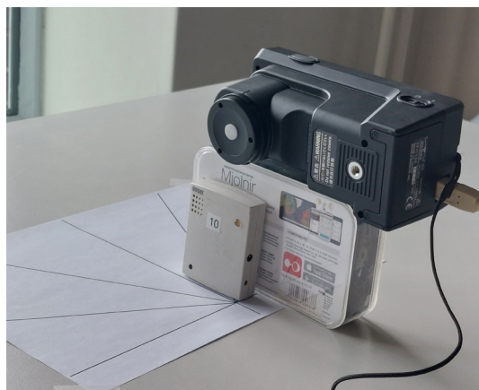
Figures 51 and 52: The setup for straight towards the window and the other angles with daylight only
