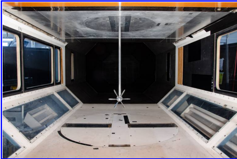
Fig. 1 Test setup (tractor configuration) installed in Delft University of Technology's Low-Turbulence Tunnel (front view).
