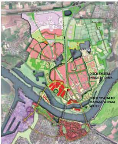
ONTWIKKELINGSBEELD 2007 development plan with elongated side channel and self-supporting water system for rain and seepage water harvesting in the Plassen (the rain water reservoirs) 4
