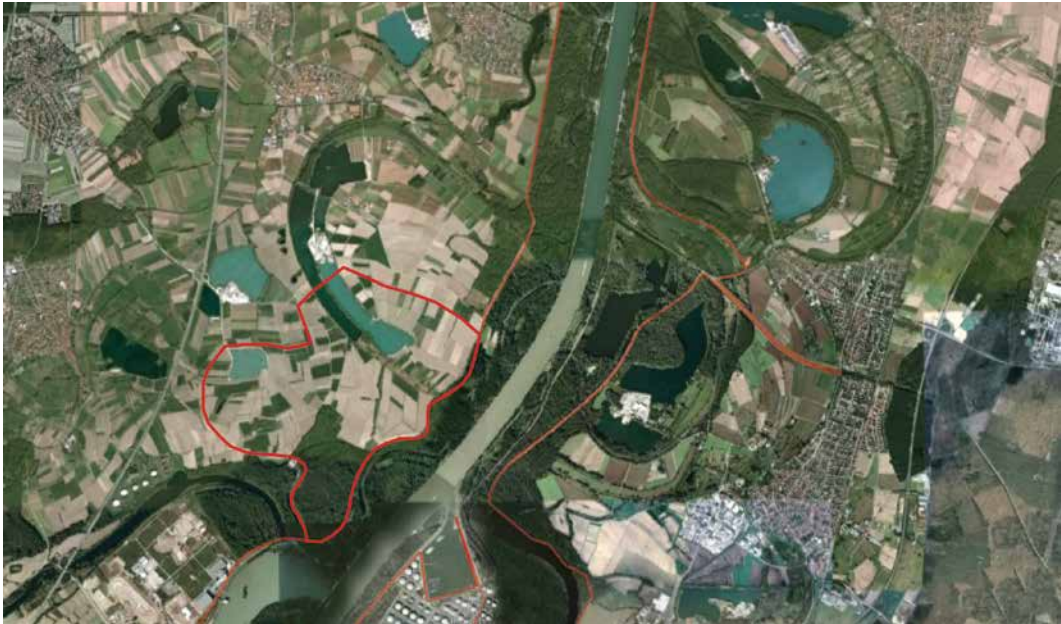
Figure 64 Neupotz Wörth (Jockgrim) Retention polder and dike set back / Rhine km 368
