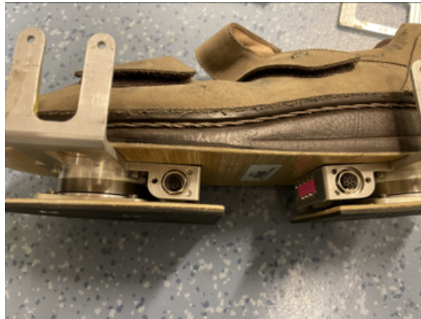
Figure D.2: Sandals with two force-torques sensors below the sole
