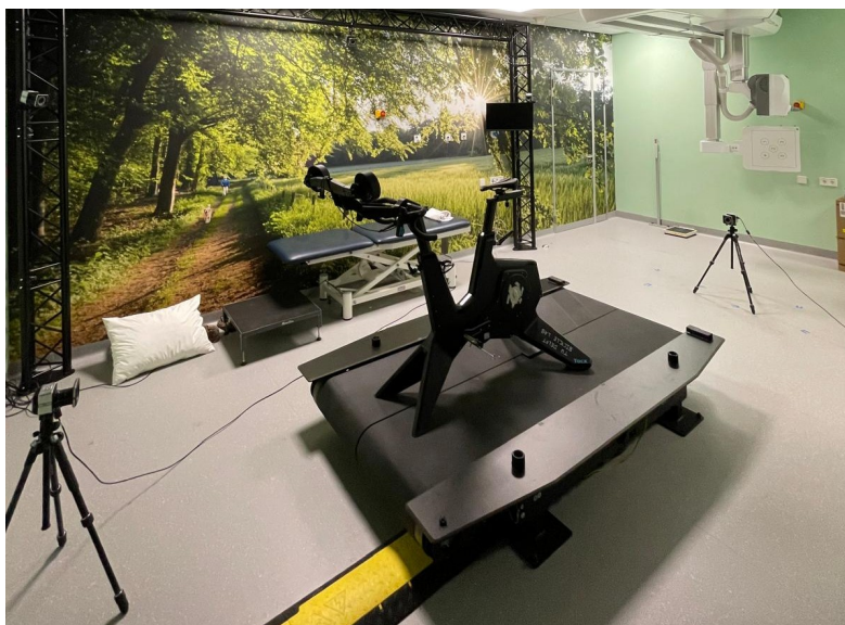
Figure D.1: Cycling setup with the bike on the treadmill, and two motion capture cameras are mounted on tripods: one in front and one behind the bike
