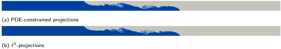
Figure D.5: Lock exchange: density field at the mesh at t^* = 10 using \ell^2 or PDE constrained particle-mesh projections. Note the different time scales used for the PDE-constrained projections and the local \ell^2 -projections.
