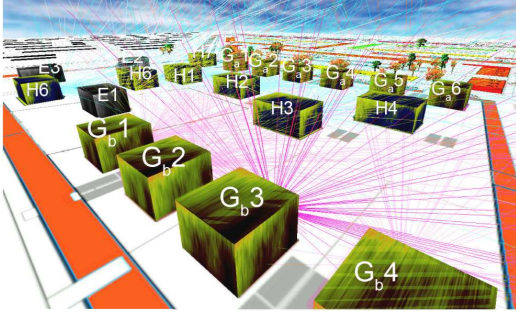
Figure 9: Illustration of the visual privacy computation based on the probabilistic perception model.
