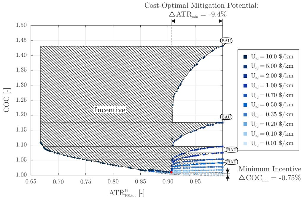
**Fig. 10** Influence of the climate unit charge ( $U_{c,j}$ ; shades of blue) on the mitigation potential of climate-charged airspaces (CCA) for the transatlantic route LIS-MIA and a threshold value ( $c_{thr}$ ) of 0.664
