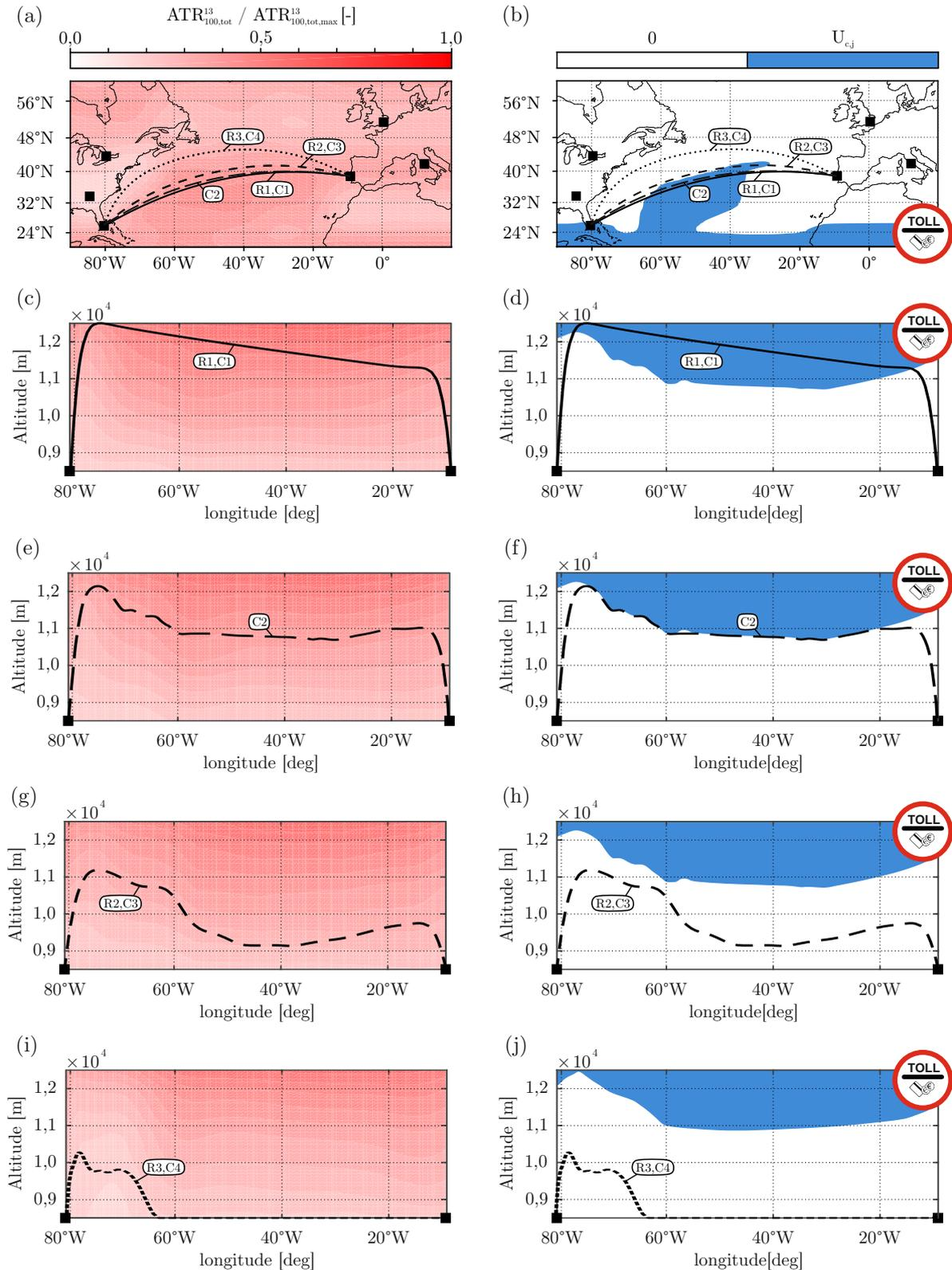
**Fig. 5** Lateral and vertical flight profiles on the North Atlantic route from Lisbon, Portugal (LIS) to Miami, USA (MIA). Contour lines of total climate change functions ( $CCF_{tot}$ ; shades of red) and climate-charged areas (CCAs; blue tone) are plotted for horizontal (top row) and vertical cross-sections (all other rows) and a threshold value ( $c_{thr}$ ) of 0.664
