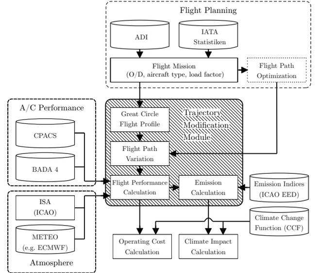
**Fig. 3** Overview of the *Trajectory Modification Module* (TMM) [4]
