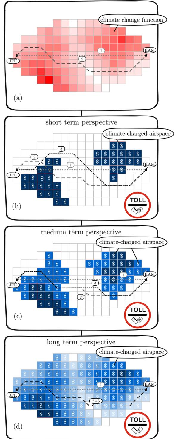
**Fig. 1** Concept of climate-charged airspaces (CCA): creating a financial incentive for airlines to minimize flight time and emissions in highly climate-sensitive regions: (1) time-optimized, (2) climate-optimized trajectory and (3) cost-optimized trajectory within the CCA concept [4]
