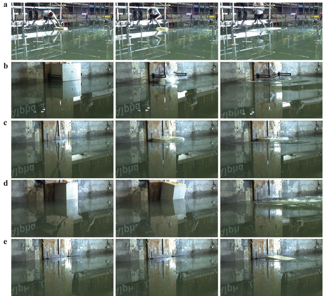
Figure 2. Image series of our large-scale experiments conducted in the basin at a water depth of 1.00 m. (a) Capsizing (mechanism A). (b) Gravity-dominated fall (B). (c) Buoyancy-dominated fall (C). (d) Gravity-dominated overturning (D). (e) , Buoyancy-dominated overturning (E). The shown examples of mechanisms A and E were conducted with a 0.800 \text{ m} \times 0.500 \text{ m} \times 0.250 \text{ m} block (type 2) and the two examples of mechanisms B, C and D with a 0.800 \text{ m} \times 0.500 \text{ m} \times 0.500 \text{ m} block (type 1). Wave profiles and movies for the five mechanisms are shown in Fig. 4 and the Supplementary Information.
