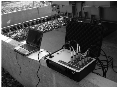
Figure 5.3 Transformer diagnostic system described by [12] during DRM field testing. The system is remotely controlled by a laptop.
