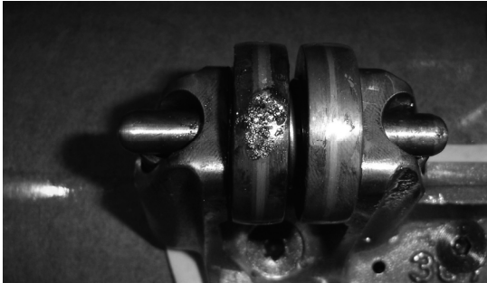
Figure A.12 Change-over selector stator roller contacts are damaged in the advanced stage of the long-term effect.
