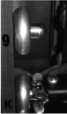
Figure 6.29 Change-over selector contact of a diverter switch type tap changer. Two contact terminals for (pre) selecting a transformer winding are shown. The bottom terminal has been selected.
