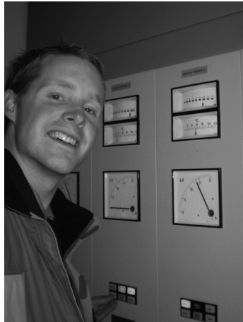
Switching the OLTC during a dynamic resistance measurement
