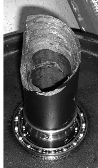
Figure A.16 Broken drive shaft of the selector switch.
