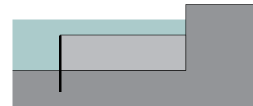
fill up behind dam; hard transition, man-made
