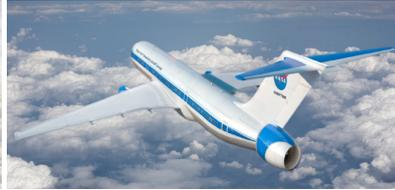
Figure 1.5: Graphical representation of NASA's STARC-ABL concept [61].
