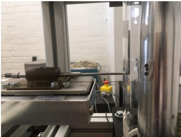
Figure 3.5: Axial traversing system in uninstalled fan test rig.
