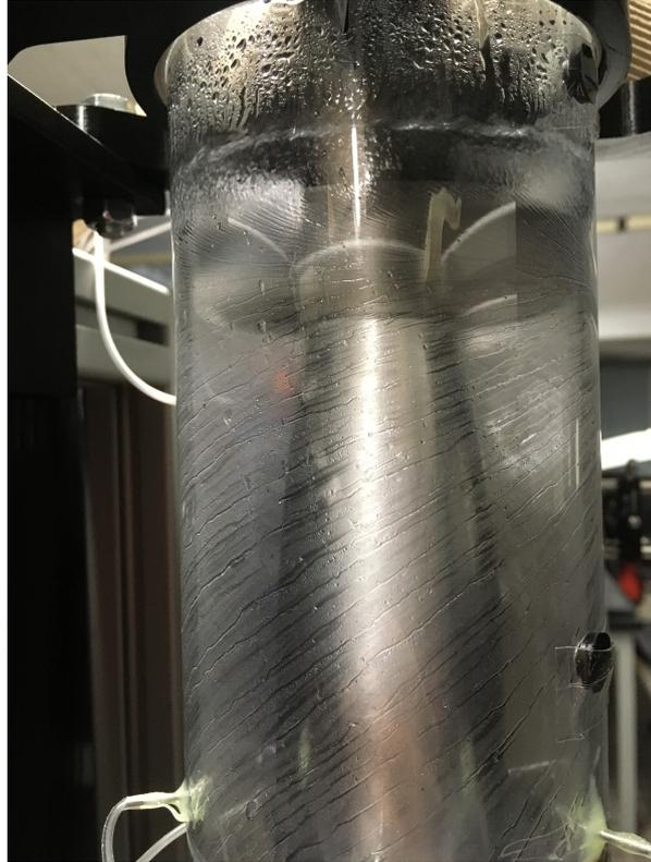
Figure A.8: Indication of flow reversal upstream of the fan.
