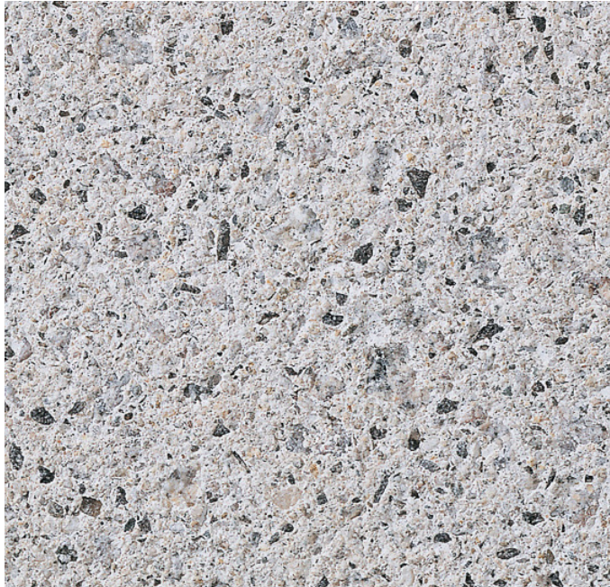
Fine exposed aggregate finish
