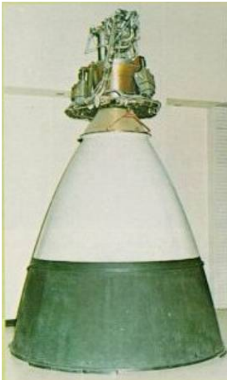
Figure F-3: Picture of the AJ10-137 engine, source: [17]
