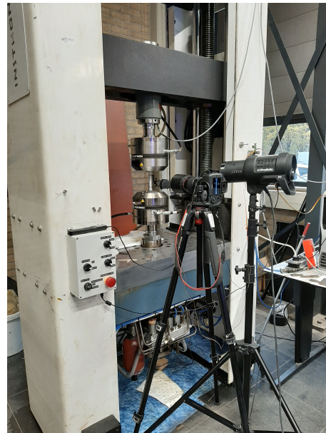
(b) Camera and flash for 2D DIC
