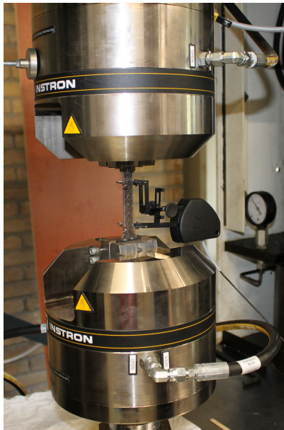
(a) Tensile coupon with extensometer
