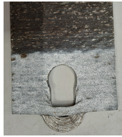
(a) Tested thin sample with paint on oxide layer
