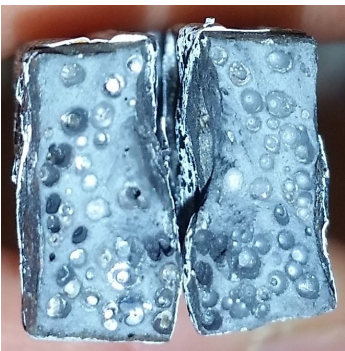
Figure M.1: Pores in tensile coupon
