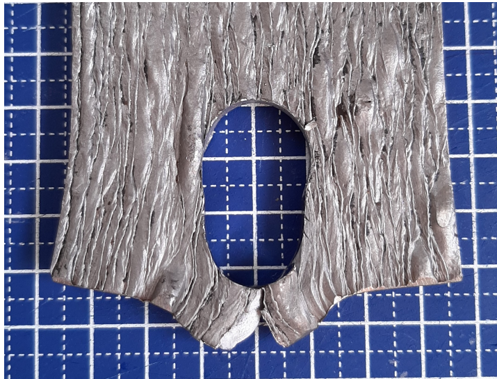
Figure L.1: Tensile failure of longitudinal thick tear-out specimen
