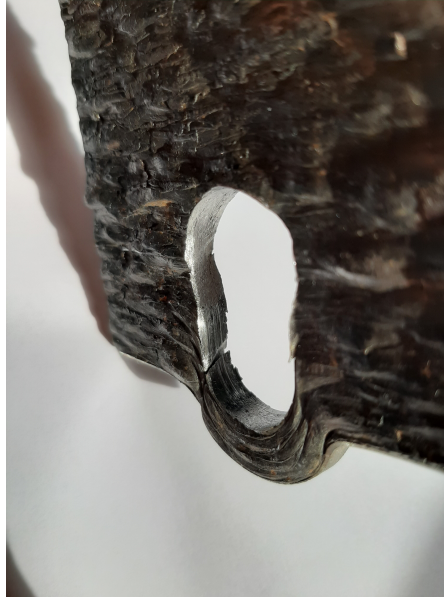
Figure 5.14: Fracture line thick transversal tear-out specimen
