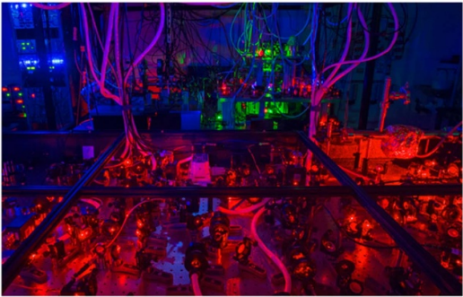
Figure 14. (Left) Atom-based experiments in quantum science like this lithium quantum gas apparatus typically utilize benchtop equipment and free-space optics which dominate the cost and complexity and restrict scalability. (Right) Properties of some atomic transitions of general interest.
