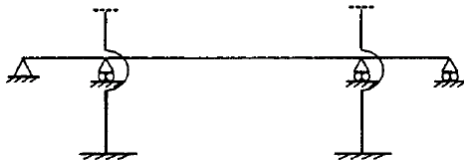
Figure 76 Supported girder in Konohana Bridge
