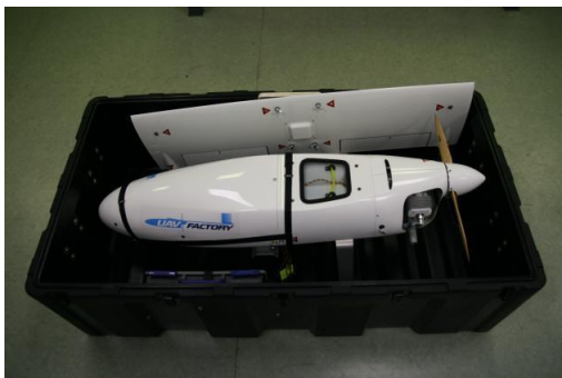
(a) Penguin B in case; 1.3 x 0.7 x 0.5 m (LxWxH) [31].
