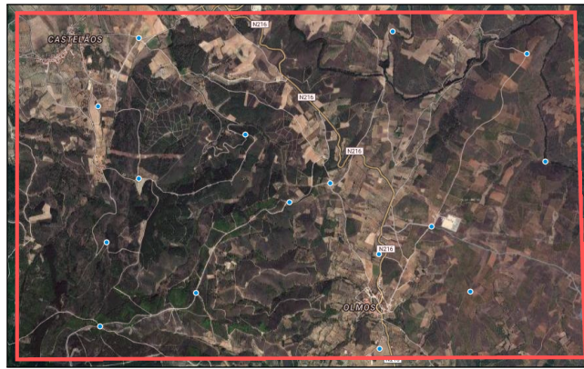
Figure 20.2: Example set of ground control points (blue dots) illustrated on a projection (pink border) of the visual camera's viewing window (6096 m x 3809 m) of a high-risk area of Northern Portugal shown in Google Maps.
