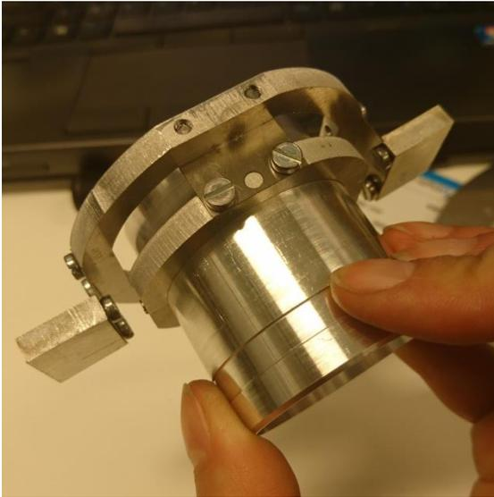
Rings for motion in x and y, attached to the fixation tube
