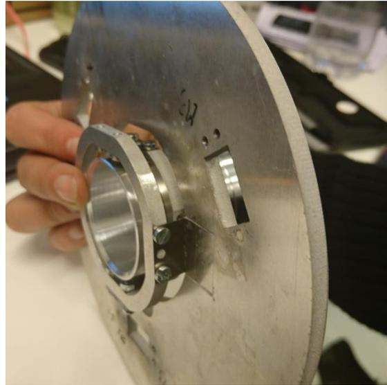
x-y platform attached to the base plate
