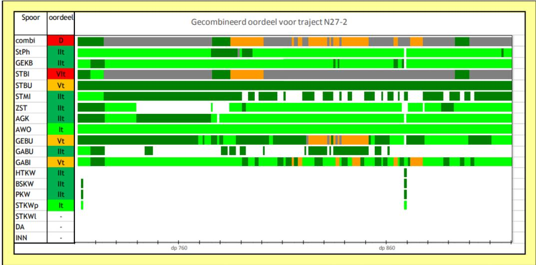
Figure A.3: Failure mechanisms assessment dike 27-2 stretch one [23]
