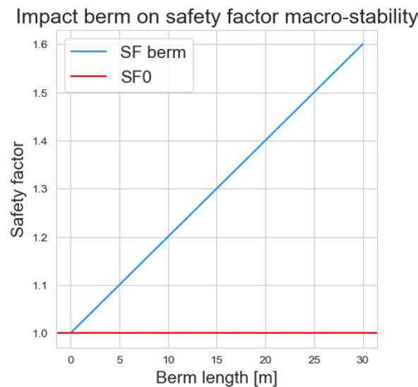
Figure 5.14: Safety factor due to construction berm
