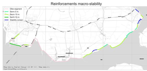
**Figure C.2:** Macro-stability reinforcements dike segment 26-3
