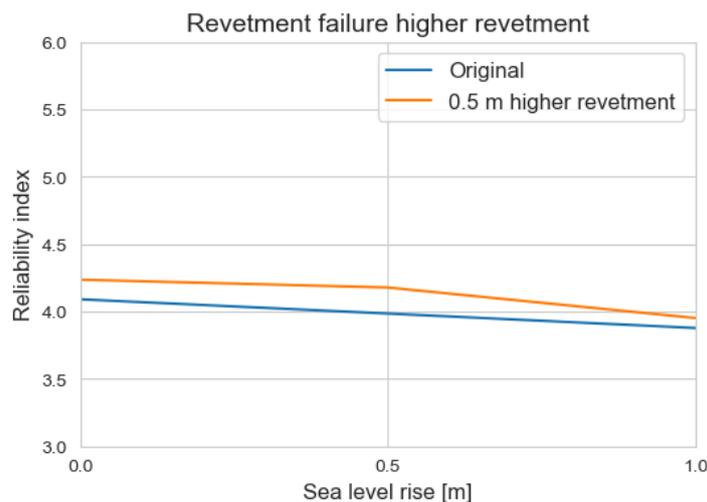
**Figure 5.16:** Revetment reinforcement impact at Bergse Diepsluis
