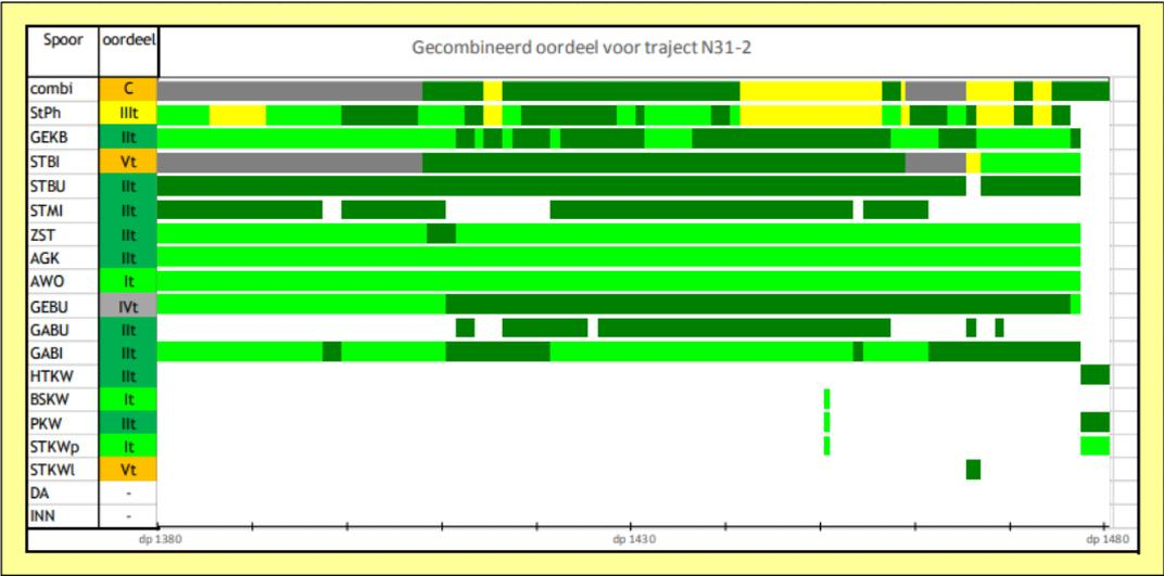
Figure A.6: Failure mechanisms assessment dike 31-2 stretch two [23]
