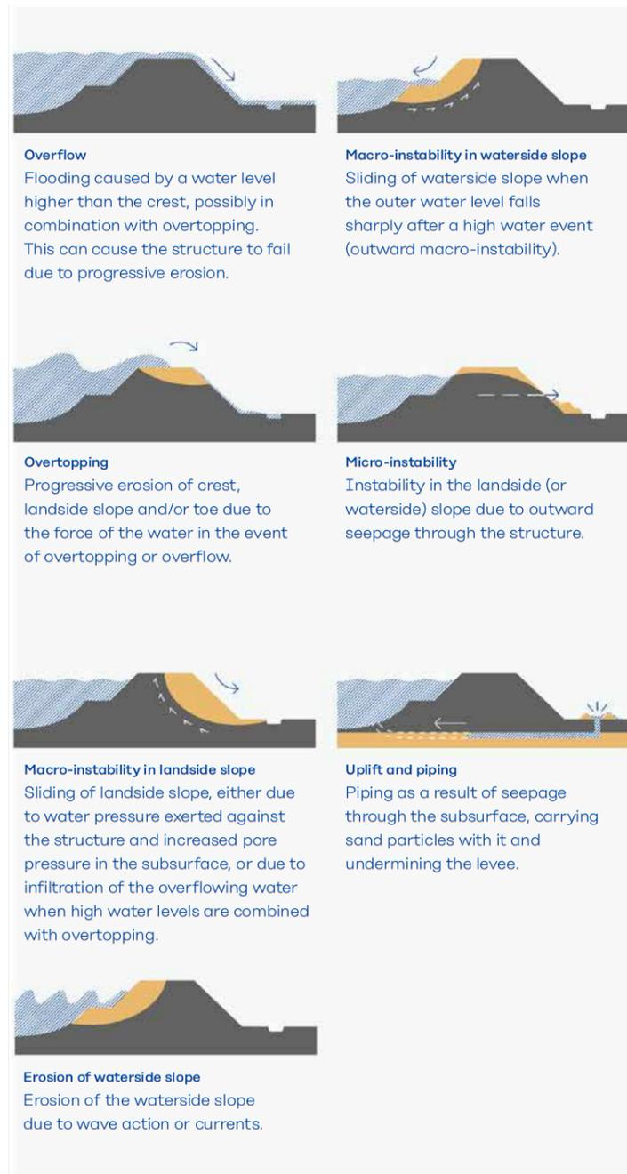
**Figure 2.6:** Failure mechanisms earthen dikes, [30]
