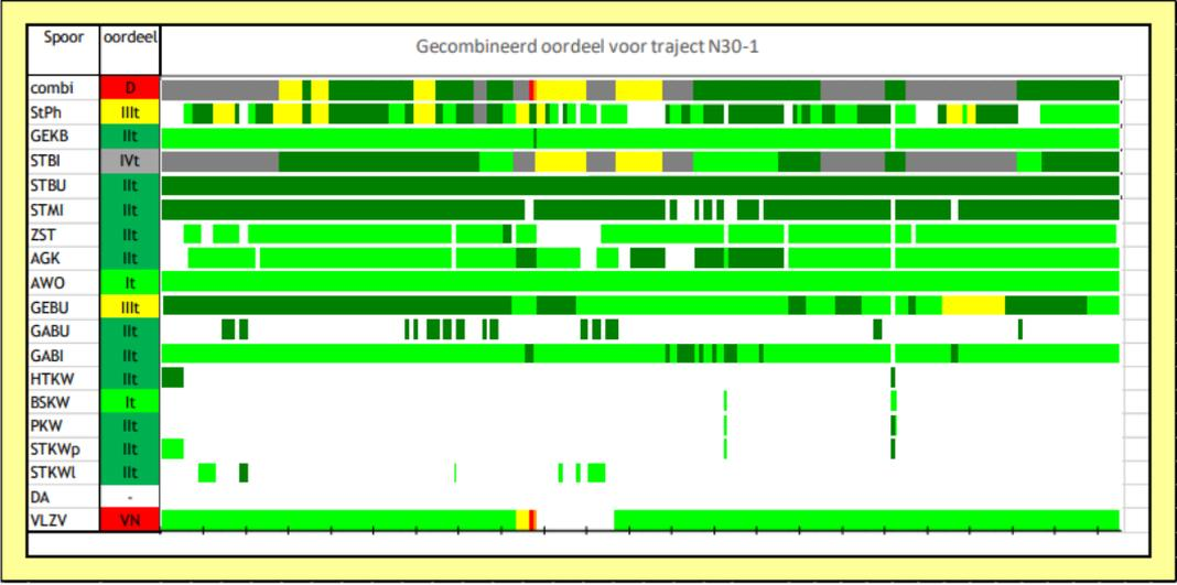
Figure A.7: Failure mechanisms assessment dike 30-1 [23]
