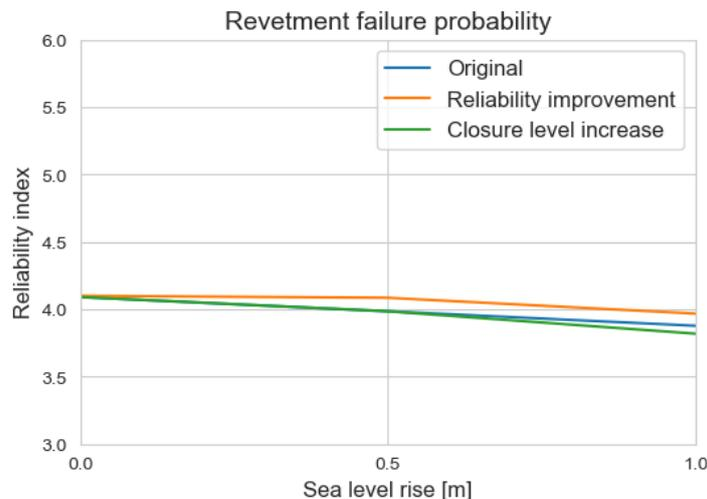
**Figure 5.18:** Revetment failure for different barrier options at Bergse Diepsluis
