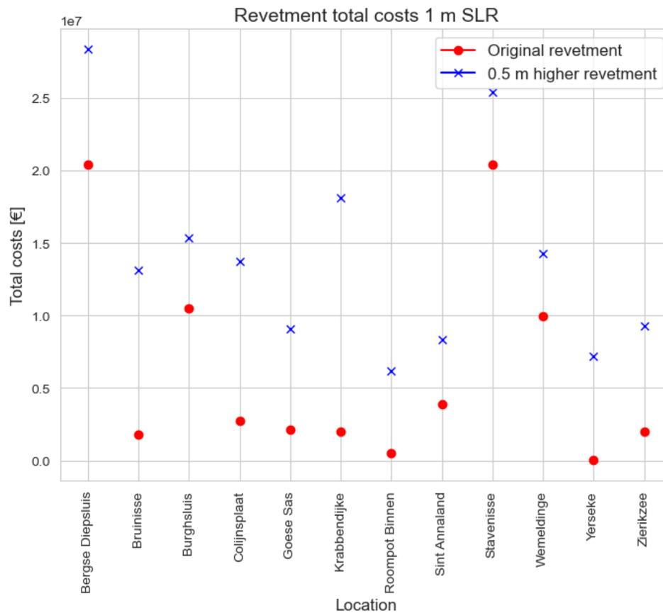
Figure 6.3: Difference costs revetment reinforcement at 1 m SLR
