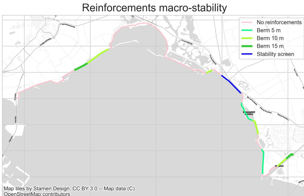
**Figure 6.1:** Macro-stability reinforcements for dike segment 26-2
