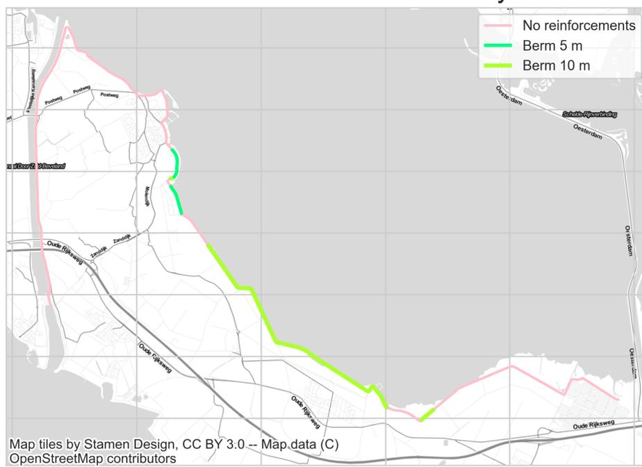
**Figure C.6:** Macro-stability reinforcements dike segment 31-2
