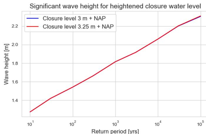
**Figure 5.2:** Wave height at Colijnsplaat for higher closure water level at 1 m SLR
