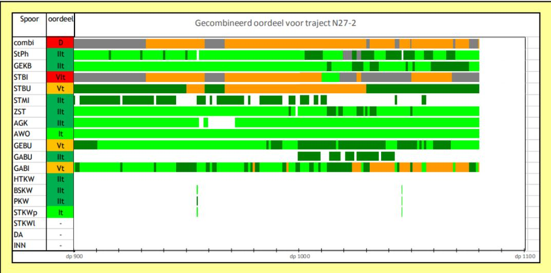
Figure A.4: Failure mechanisms assessment dike 27-2 stretch two [23]
