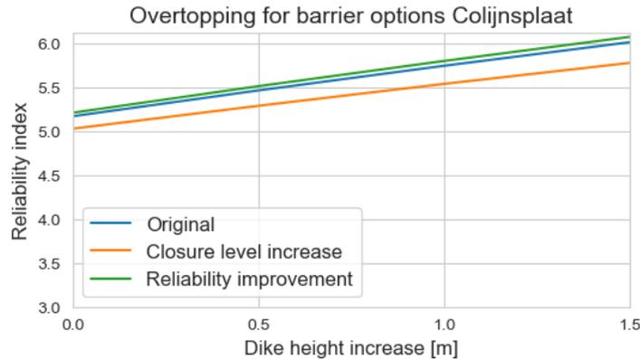
**Figure 5.17:** Overtopping reliability for different barrier options at Colijnsplaat for 0 m SLR
