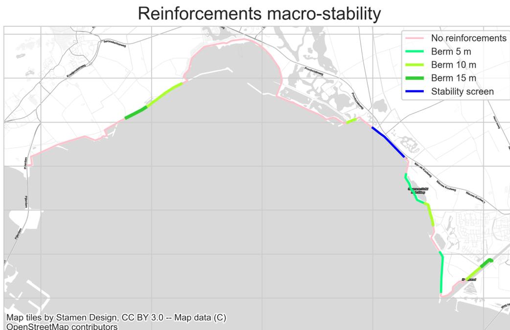
**Figure C.1:** Macro-stability reinforcements dike segment 26-2
