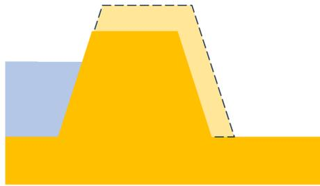
Figure 5.8: Dike heightening reinforcement schematisation
