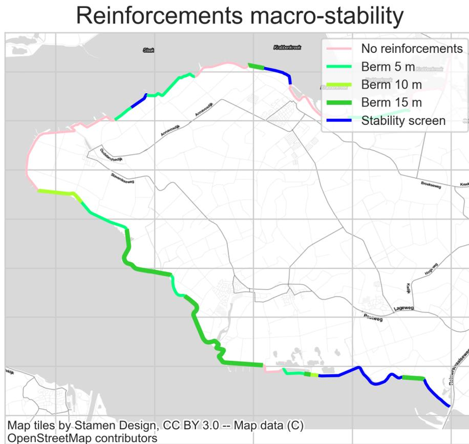
**Figure C.3:** Macro-stability reinforcements dike segment 27-2
