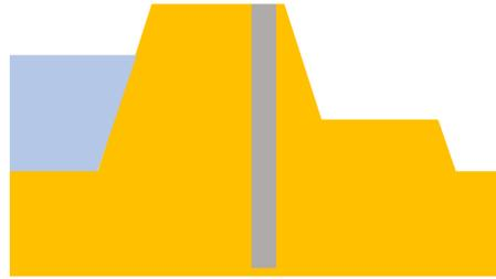
Figure 5.11: Schematisation diaphragm wall
