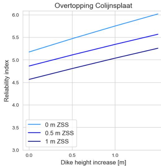
**Figure 5.15:** Heightening the dike against overtopping failure
