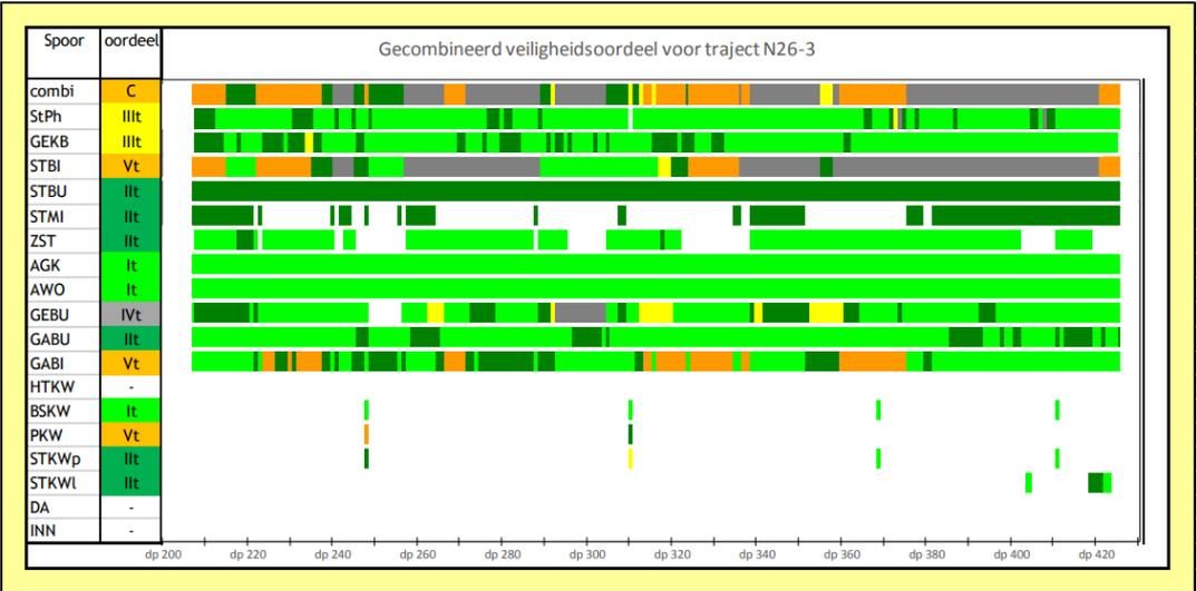
Figure A.2: Failure mechanisms assessment dike 26-3 [23]
