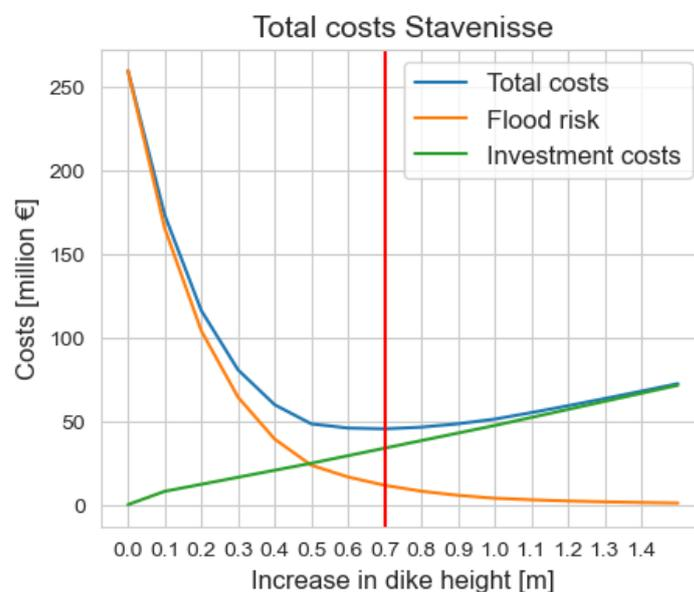
**Figure 6.6:** Costs for Stavenisse for 1 m SLR and heightened closure water level
