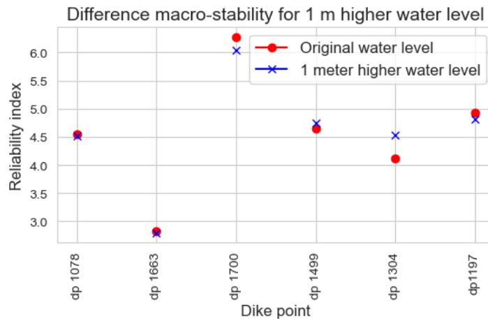
**Figure 5.9:** Change in reliability index macro-stability for 1 meter higher water level
