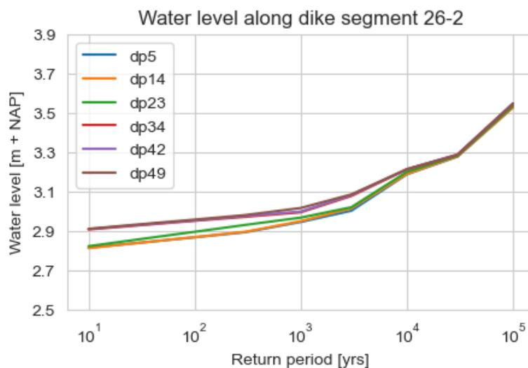
Figure 5.5: Water level along dike segment 26-2
