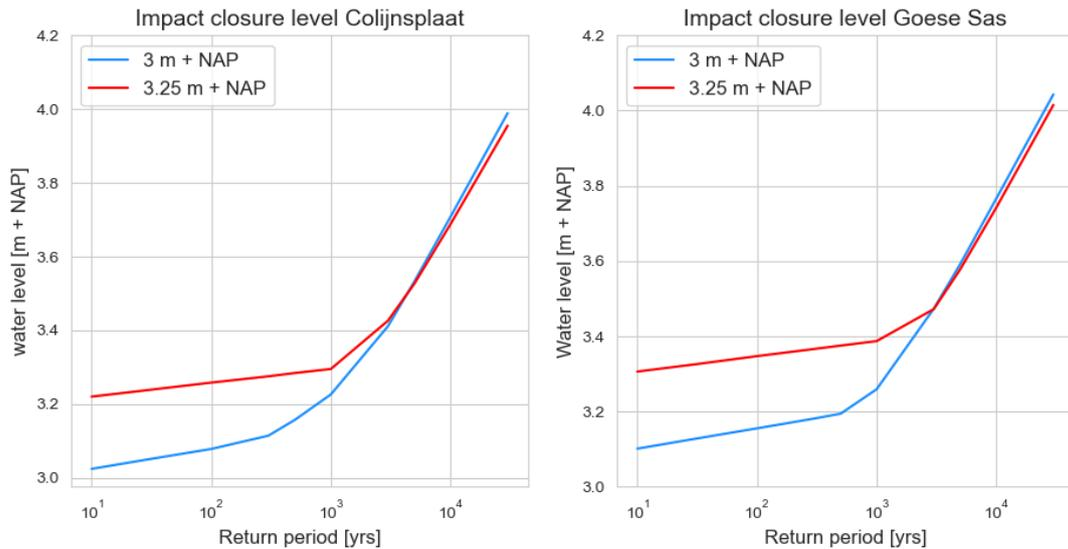
**Figure 5.1:** Effect of 25 cm higher closure water level at 1 m SLR
