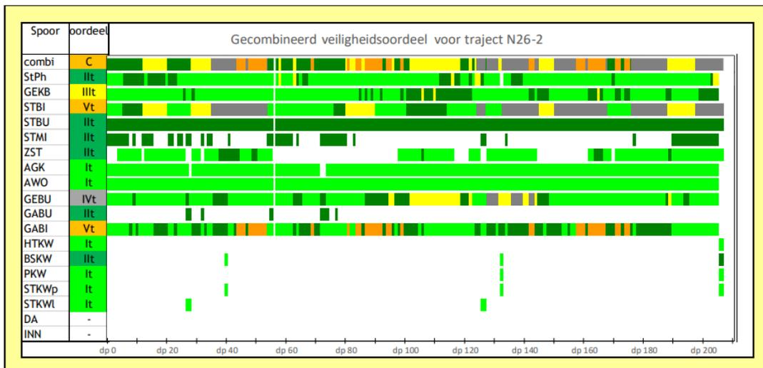
**Figure A.1:** Failure mechanisms assessment dike 26-2 [23]
