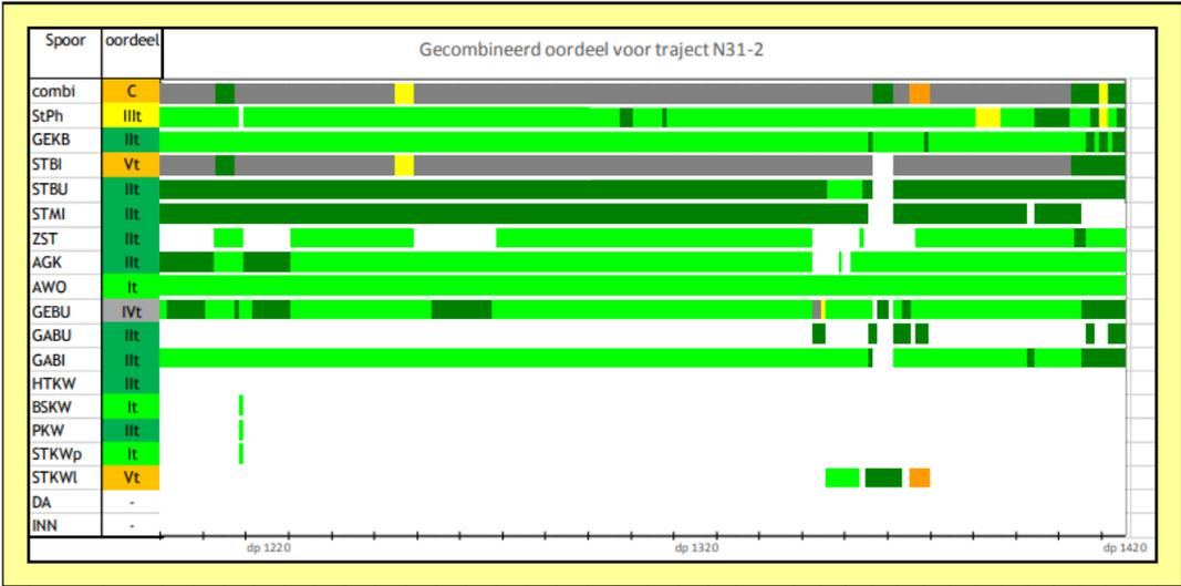
Figure A.5: Failure mechanisms assessment dike 31-2 stretch one [23]
