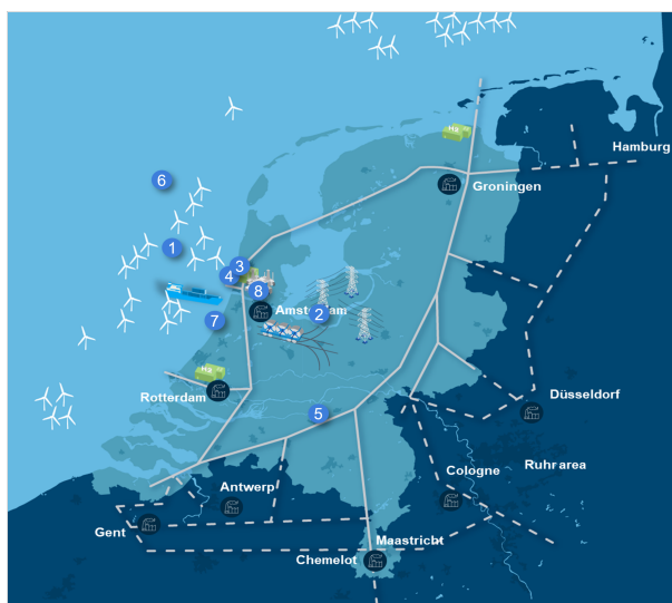
Figure 5.4: Visual representation of the hydrogen backbone in the Netherlands. 1: Offshore wind energy, 2: High-voltage grid connection, 3: Connection to hydrogen backbone, 4: Importing or production of hydrogen, 5: Current gas infrastructure, 6: CCS in empty gas fields, port for importing hydrogen or exporting CO 2 . Figure obtained by Tata Steel, 2025c.
