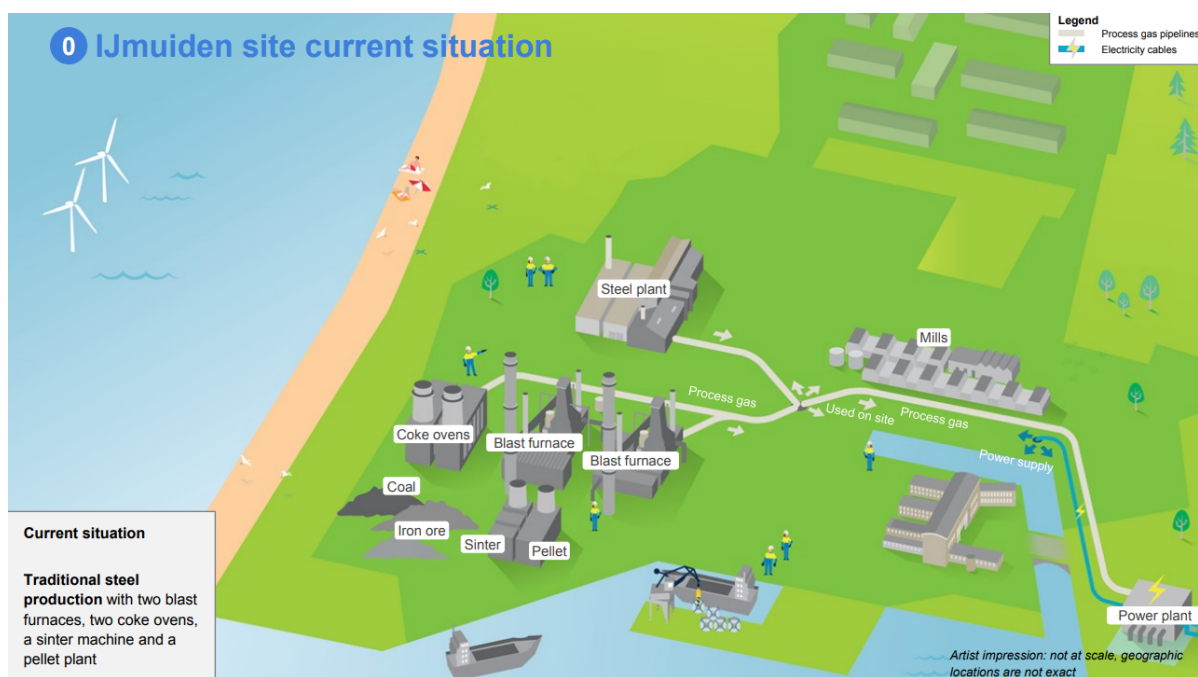
Figure D.1: Visual representation of the current iron and steel production at Tata Steel IJmuiden.
