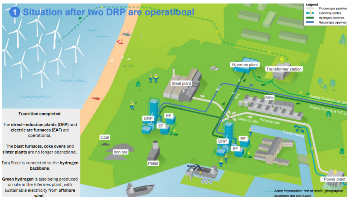
Figure D.3: Visual representation of the decarbonized iron and steel production at Tata Steel IJmuiden.
