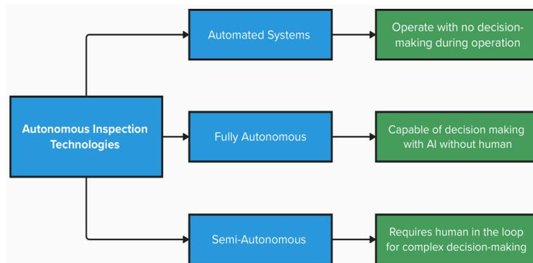
FIGURE 6. TYPES OF AUTONOMOUS INSPECTION TECHNOLOGIES
