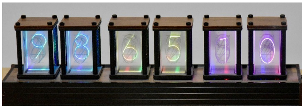
Figure 15. Modern numeric display device using LEDs
