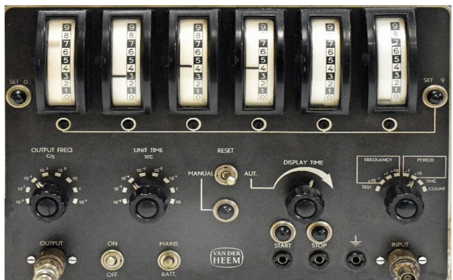
Figure 6. Transistorized counter by Van Der Heem using analogue meters for display
