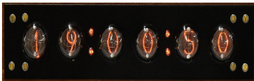
Figure 11. Electronic clock, which uses Nixie-tubes, displaying '19:00:50'
