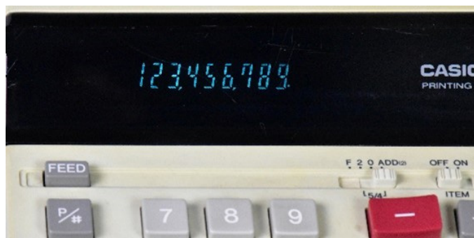
Figure 12. Casio FR 310 Printing Calculator using seven-segment indicators
