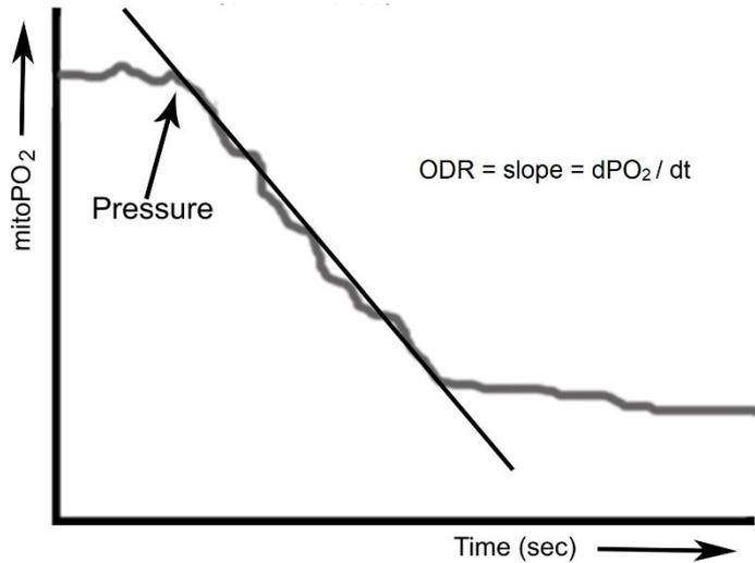
**Figure 1:** Principle of mitochondrial oxygen consumption (mitoVO<sub>2</sub>) by pressure-induced occlusion of the microcirculatory blood flow. MitoVO<sub>2</sub> is calculated from the linear part of the oxygen disappearance curve. Printed from: Harms et.al. (1)
