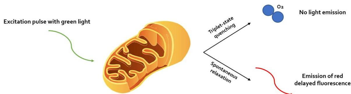
**Figure 2:** Principle of the protoporphyrin IX (PpIX)-triplet state lifetime technique. After an excitation pulse with green light, PpIX possesses an excited triplet and causes the emission of red delayed fluorescence. However, the excited triplet state reacts strongly with oxygen. Collision with an oxygen molecule is called triplet-state quenching. Triplet-state quenching results in the relaxation of PpIX without light emission.
