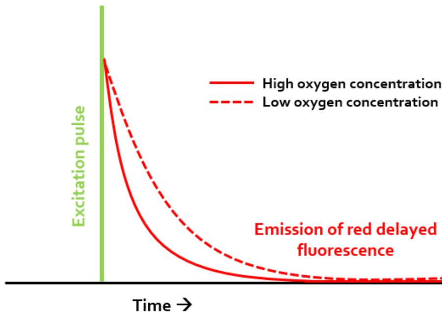
**Figure 3:** Protoporphyrin IX (PpIX) emits red delayed fluorescence after excitation by a pulse of green light. The delayed fluorescence lifetime depends on the oxygen concentration in the mitochondria. High oxygen concentration will increase the collision frequency. Collisions of PpIX with oxygen will shorten the delayed fluorescence lifetime.
