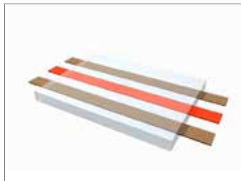
Figure 6.3i Recovery is fixated by cooling SMP body
