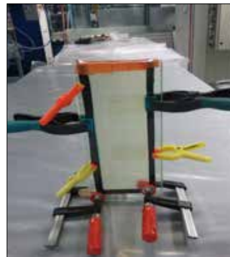
Figure 7.28 Glass mould with cured SMP.
