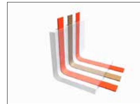
Figure 6.3d SMP is cooled to fixate the deformation
