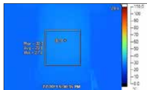
Figure 8.7a Thermal image activation constantan, U=15\text{V} t=0\text{s}
