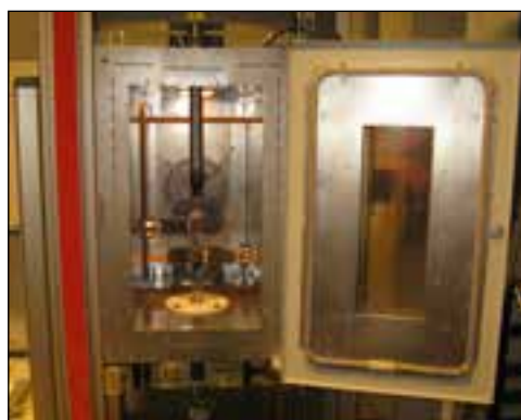
Figure 7.5 Zwick Roell Z005 torsion bench with heating chamber.
