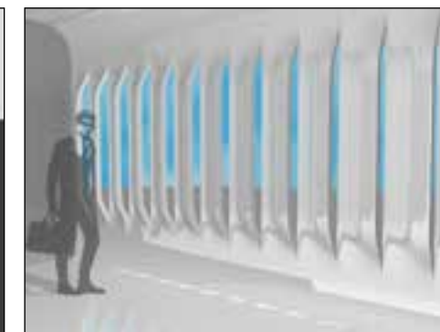
Figure 4.7 Vertical lamella system for ventilation purposes
