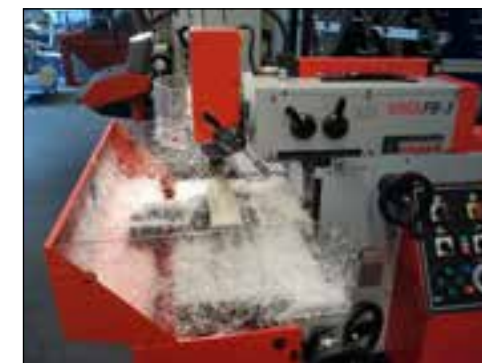
Figure 7.29 Milling of the SMP body.
