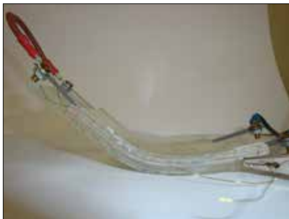
Figure 7.49 Prototype with full integration of heating wires. The SMP is 80*60 mm, the SMAs maintain similar dimensions. A recovery of 135° is reached.
