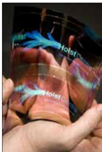
Figure 3.17 OLED can be wrapped and stretched without degradation. Image courtesy by Holst Centre.
