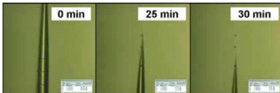
Figure 3.5 Time dependent crack closure in polymer. Image courtesy Fraunhofer UMSICHT
