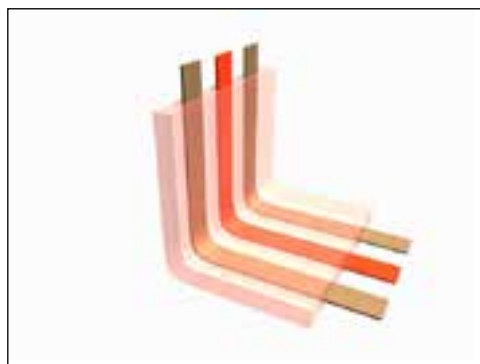
Figure 6.3g SMA 2 is heated to initiate recovery
