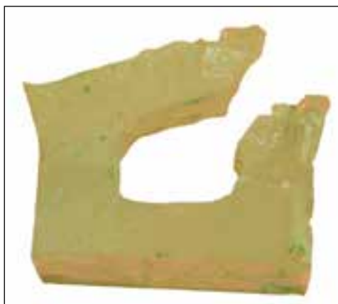
Figure 7.39 SMP specimen. The super glue gives a strong bond and the SMP ruptures.
