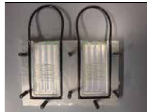
Figure 7.33 Second fabrication method for the integration of the heating wires in the SMP matrix. First, one part of the SMP is partly cured. Then the wires are glued in the required pattern. Third, the other part of the SMP is casted and the whole SMP is fully cured.
