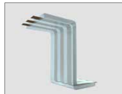
Figure 7.26 Smart Composite that facilitates the deformation at two locations of the component body
