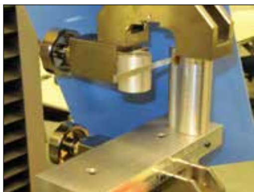
Figure 7.22 Research setup martensite deformation SMA strip
