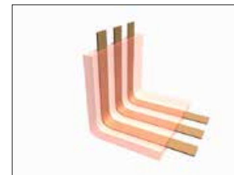
Figure 6.3f SMP is heated, until it reaches the fully rubbery state
