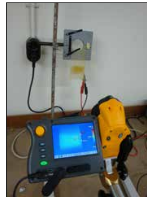
Figure 8.6 Research set-up of the thermoelectric activation of the SMP
