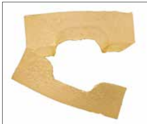
Figure 7.37 SMP specimen. The Araldite 2015 shows rupture of the bonds.
