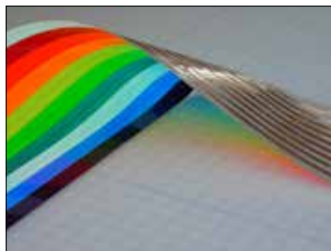
Figure 3.18 EL light strip. Image courtesy Earlsmann.
