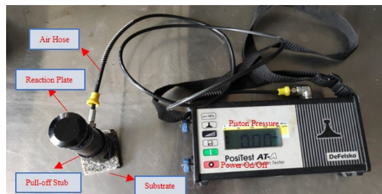
Figure 4. ASTM D 4541 Type IV adhesion tester.
