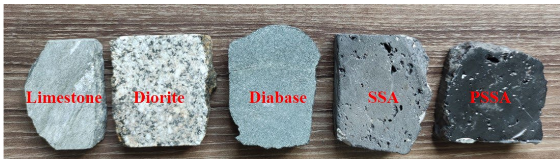
Figure 3. Aggregate samples for BBS test.
