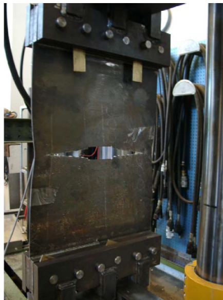
Figure 30: Test specimen after failure [51].
