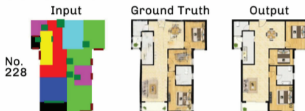
Figure 3.8: The machine learning based method for space layout generation as implemented by (W.Huang, n.d.)
