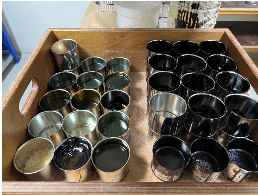
Figure 3. Rejuvenators (left part) and rejuvenated bitumen samples (right part) made in this project.
