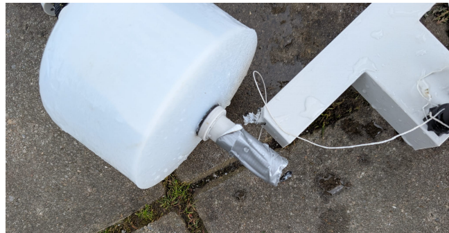
Figure D.4: Breaking point (with unsuccessful duct tape as a solution)
