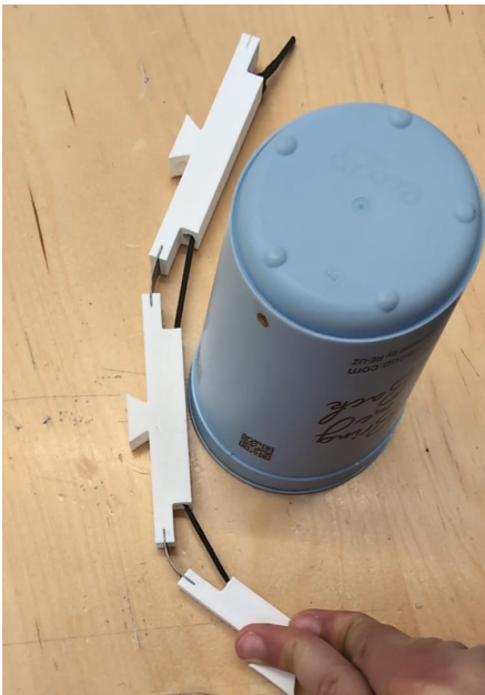
Figure 2.3: First gripper prototype, with an overall arm length of 300 mm.
