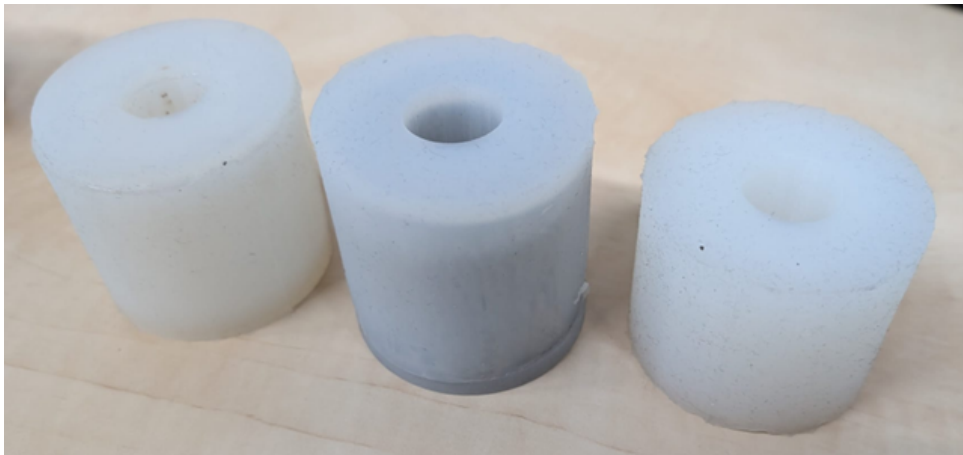
Figure 2.9: Flexible wheel prototypes with varying internal media, measuring approximately 60 mm in diameter and 60 mm in height. From left to right: water-filled, granular-filled, and solid silicone variants.
