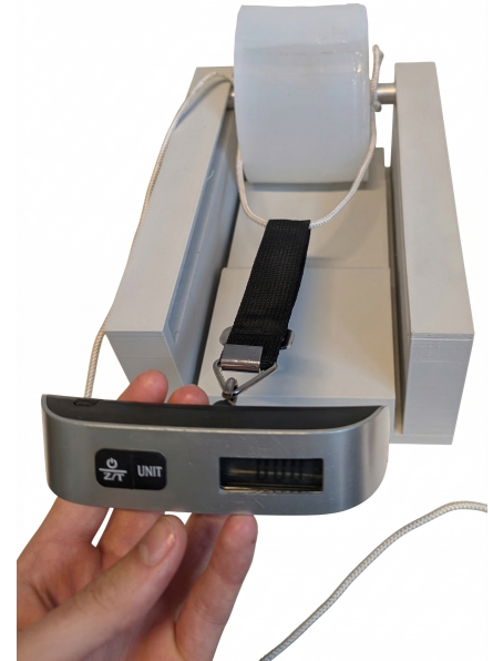
Figure 4.2: Friction measurement setup used for empirical model calibration.
