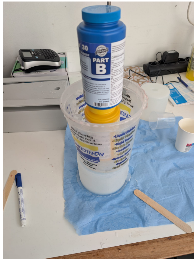
Figure B.1: Joining top and bottom of the wheel, with bottles as weights to ensure proper sealing.
