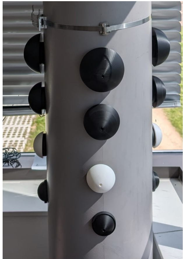
Figure 5.4: Experimental setup for obstacle handling, featuring a 0.3 m diameter pipe with rigid protrusions of 30, 40, 50, and 60 mm radius.
