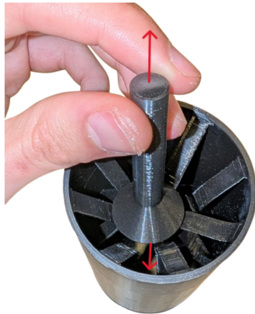
Figure 2.2: The structurally fragile compliant funnel prototype. This 60x100 mm assembly relies on an arrow-shaped rod pushing past flexible internal latches to lock. translating along the path indicated by the red arrows.
