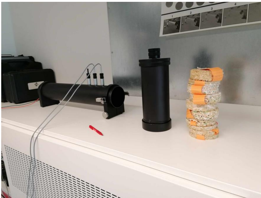
Figure 70: Impedance tube and the samples
