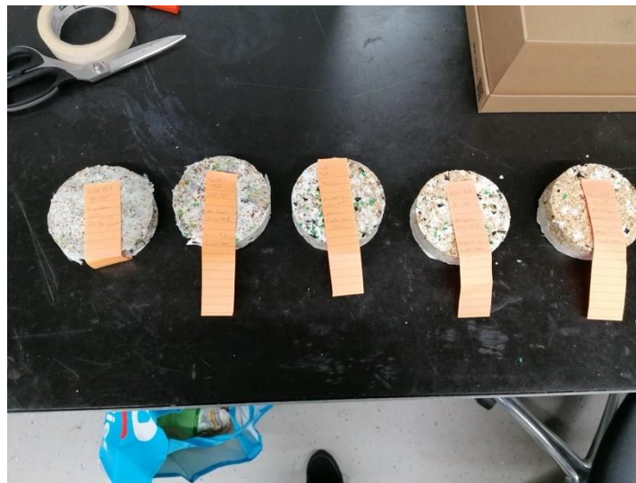
Figure 5: First set of samples with varying PLA content
