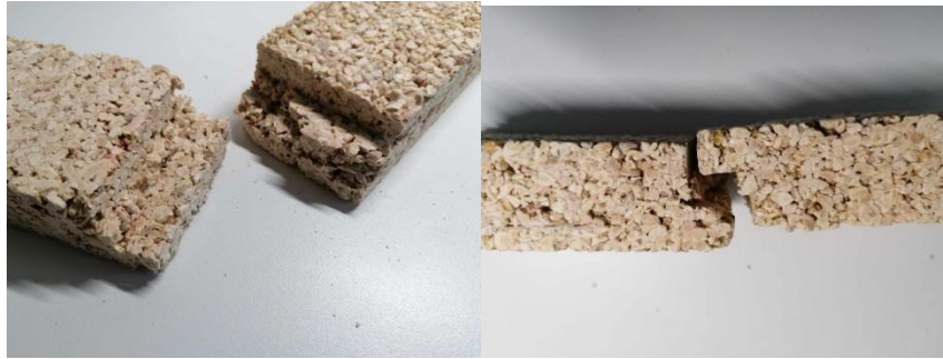
Figure 46: Edge joint sample
