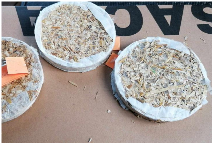
Figure 42: Corn cob and PLA samples
