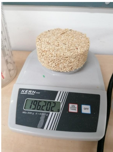
Figure 9: 3.5 cm corn cob and wood glue (15%)
