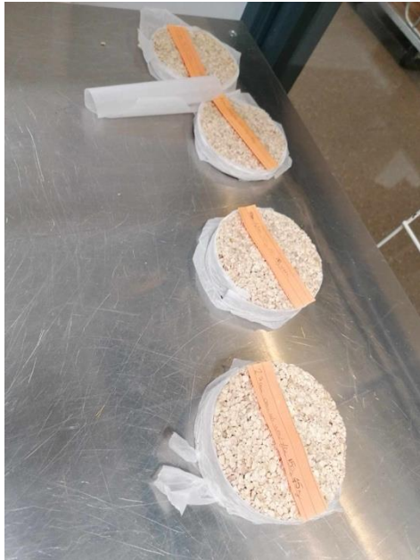
Figure 41: Corn cob and wood glue samples with varying thickness
