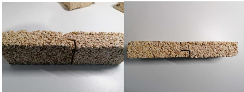
Figure 45: Lap joint sample
