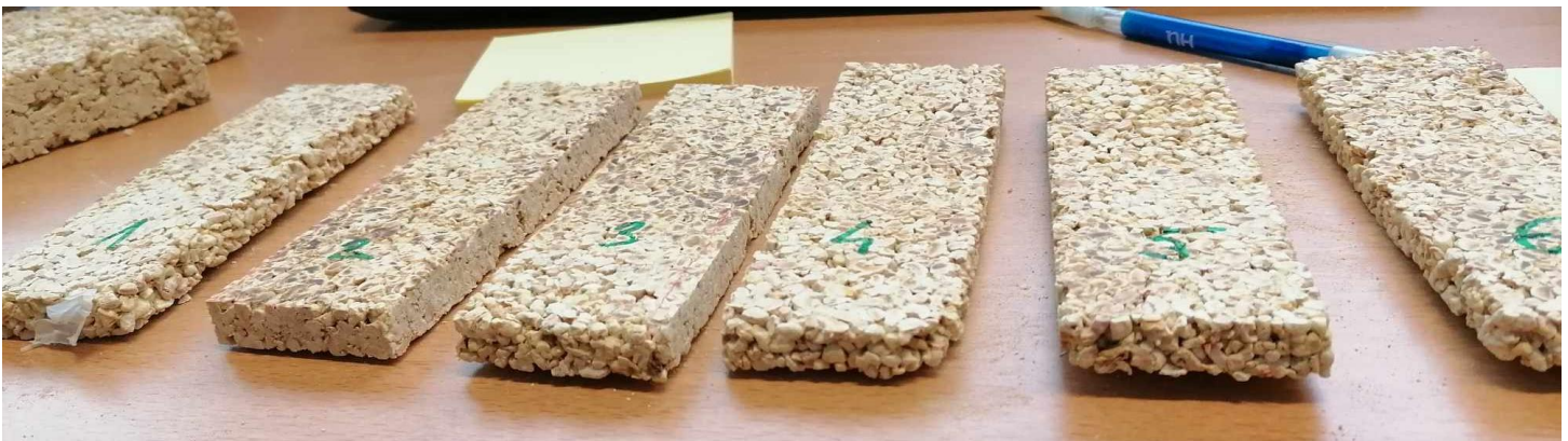
Figure 43: Samples created for the bending test
