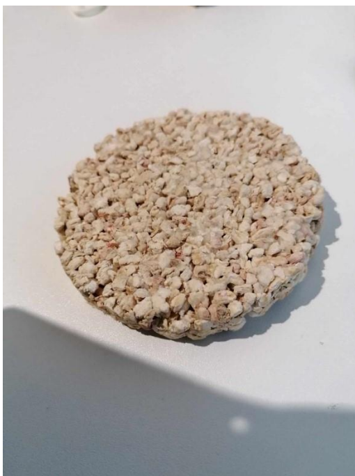
Figure 10: 1 cm corn cob and wood glue (23%)
