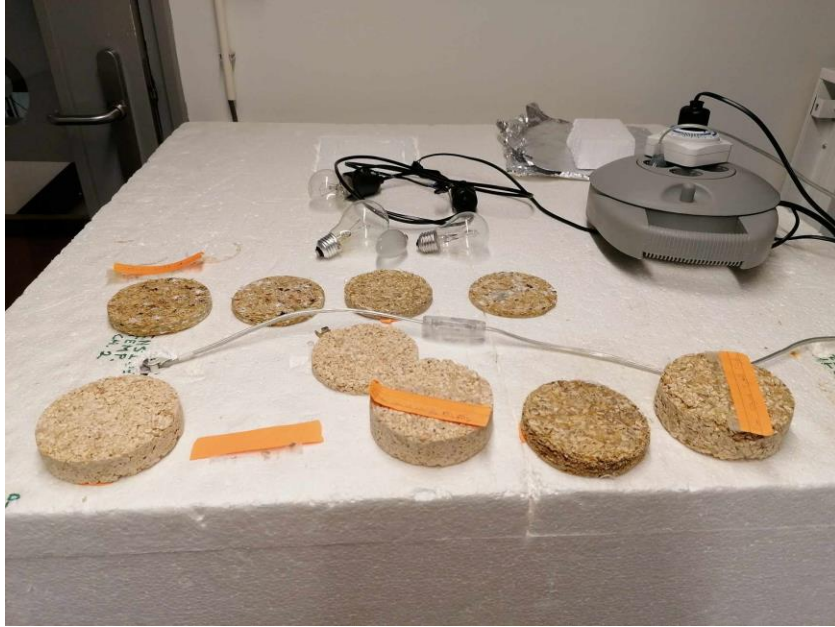
Figure 50: Samples created for the “sandwich” acoustic testing
