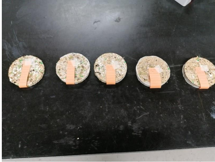
Figure 8: Finished corn cob, corn stalk and PLA samples
