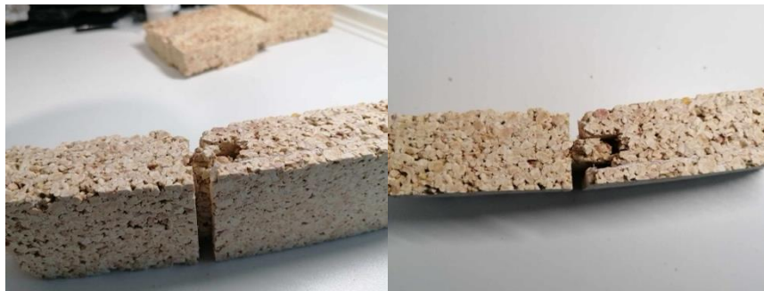
Figure 44: Tong and groove sample
