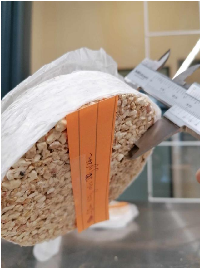
Figure 77: Corn cob and wood glue sample
