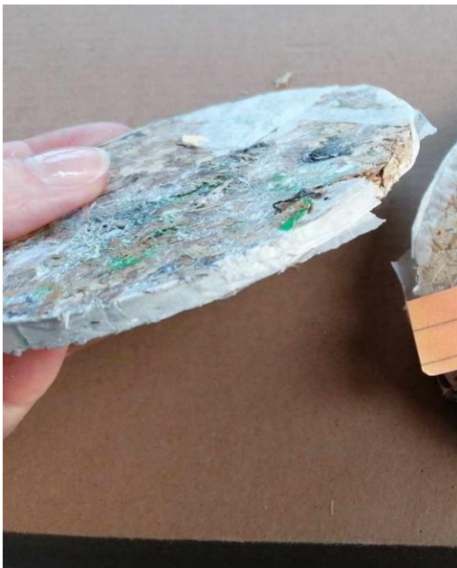
Figure 76: Sample of a 0.5 cm corn stalk and PLA sample
