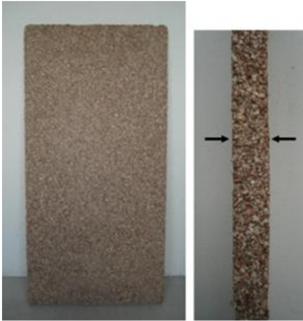
Figure 69: Sample of the corn cob board
