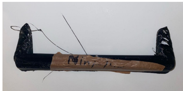
Figure 55: Failed Ninjabflex 3D print.
