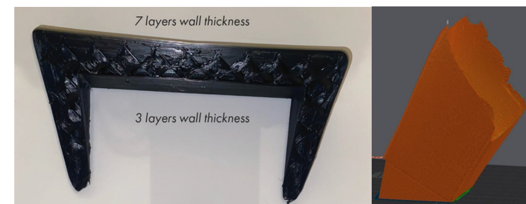
Figure 57: First Cheetah print (left) with original print orientation (right).
