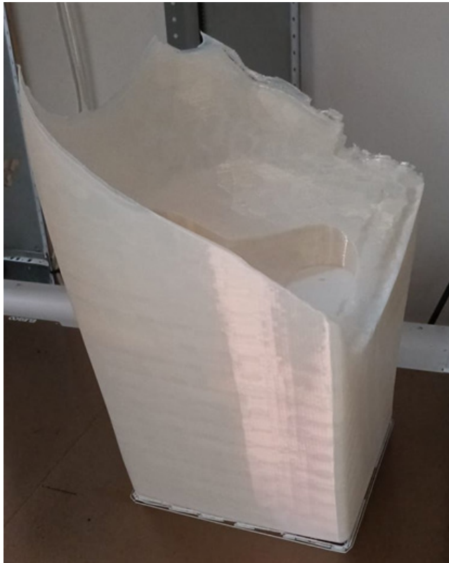
Figure 61: Final Hytrel and TPU print.
