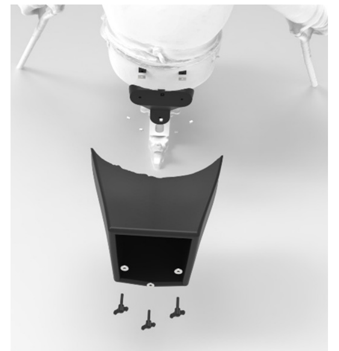
Figure 75: Exploded view of all components
