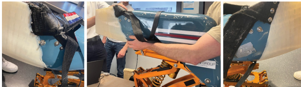
Figure 62: Test fitting the shell component, 2 times right side and left side.
