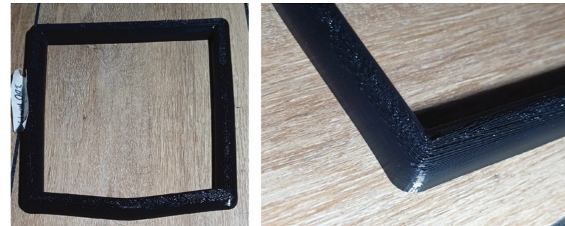
Figure 59: Support material testing with a closeup of the edge.
