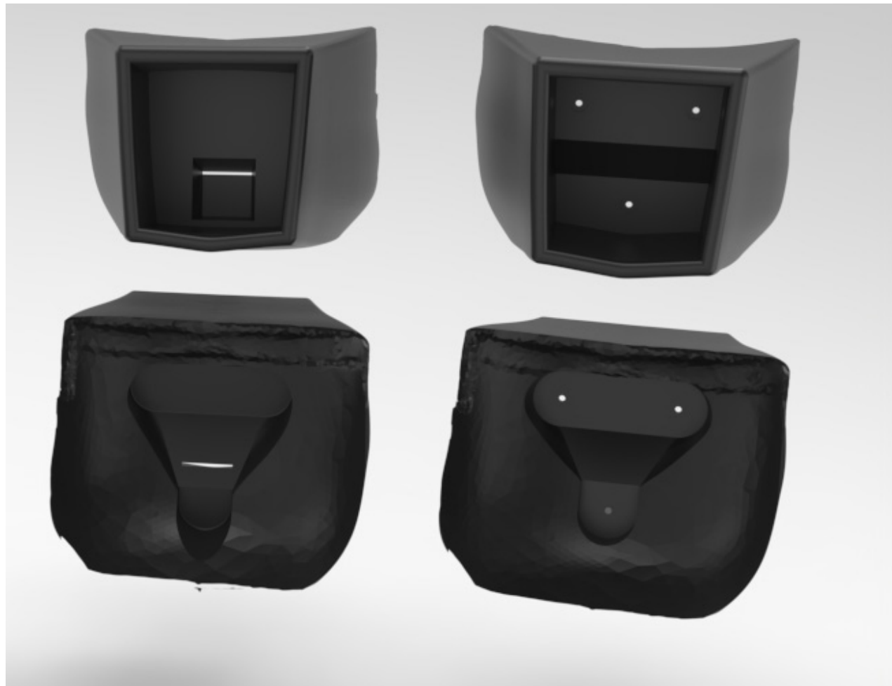
Figure 73: Final evolution of the aerodynamic shell.
