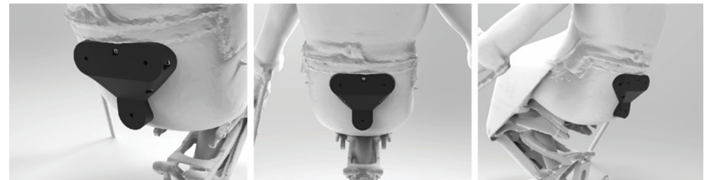
Figure 72: Final mounting plate from different angles.
