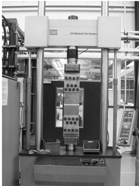
**Figure 6.2** – *TU Delft's 500 kN servo-hydraulic fatigue test machine with specimen installed.*
