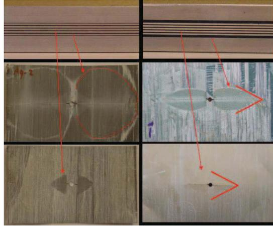
**Figure 2.2** – Comparison of delamination areas for adhesive (left) and bondpreg (right) CentrAl laminates [11]
