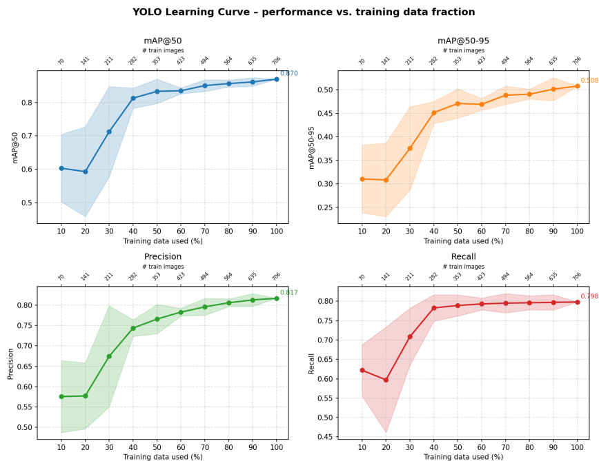
Figure 14: YOLO learning curve evaluated against the same test set with increasing proportions of training data. Five folds were used for training set selection to account for split variability; the graph shows the mean performance per split as well as the minimum and maximum. For the final 100% split, results across all five test splits were used, as these were deemed more representative of the model’s performance on unseen data.
