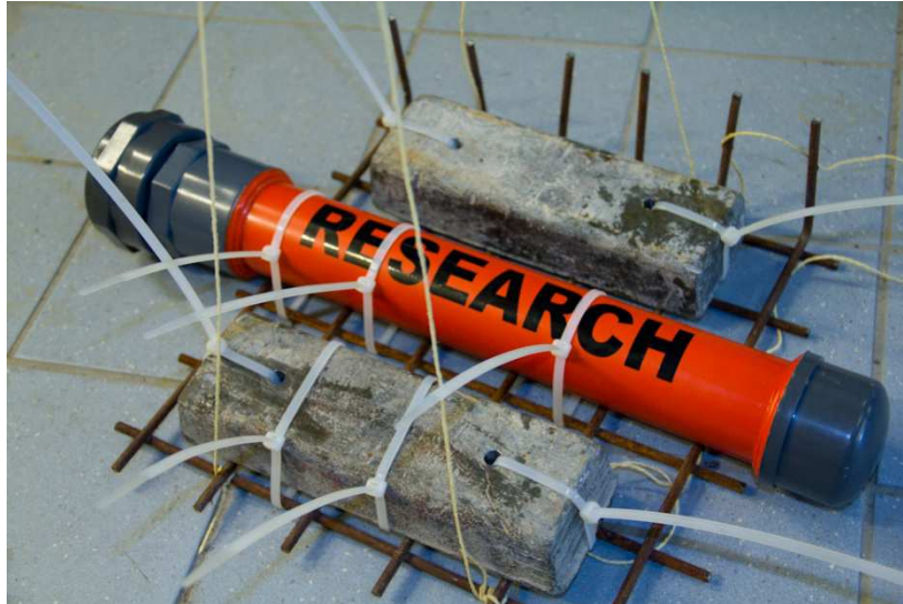
Figure 5.3 The pressure meter in combination with the lead blocks.
