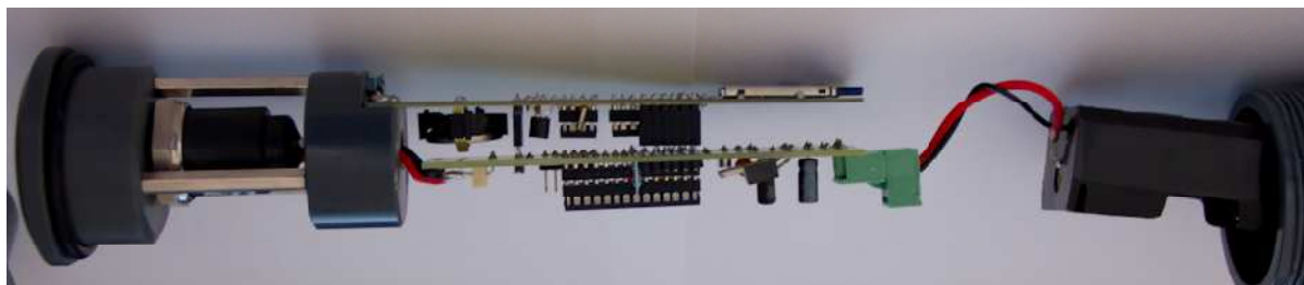
Figure 5.2 The inside of the pressure meter
