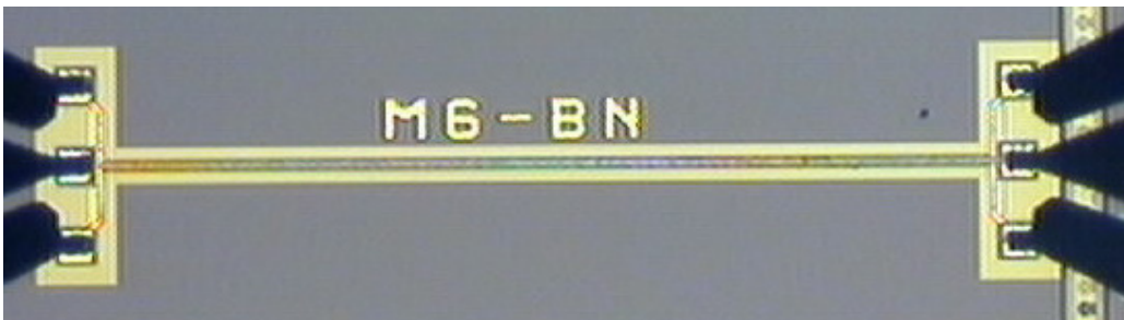
Figure 2.26: Photomicrograph of a single-ended transmission line implemented in Philips' QUBiC4G process.
