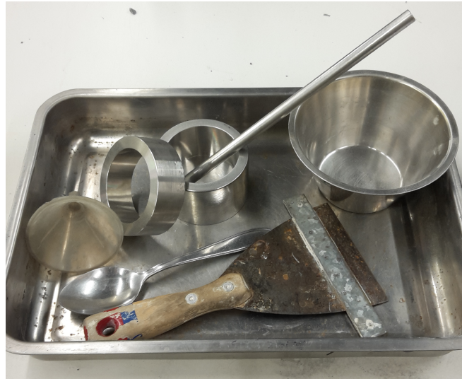
Figure C.15: Apparatus used for obtaining the maximum and minimum density of the soil based on [2]
