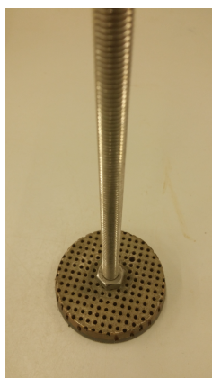
Figure C.27: Tamper used for compaction of the sand layers [23]
