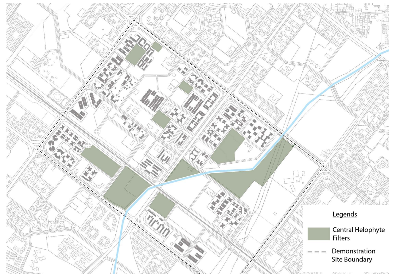
Fig 8.27: Water treatment by helophyte filters Source: Clicked by author
