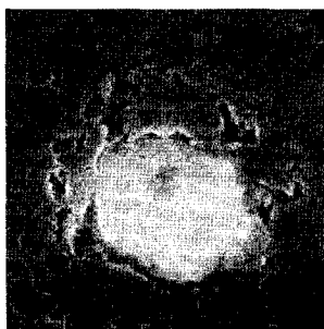
Figure 5.4: SEM micrographs of Alclad 2024 alloy after 5 minutes of immersion in the \text{H}_3\text{PO}_4\text{-H}_2\text{SO}_4 solution (sample NP).
