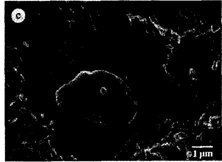
Figure 2.6: Crystallographic pit around a large intermetallic on the surface of AA3005 after 15 minutes of immersion in 5 wt.% NaCl pH=3 solution [Ref. 66].
