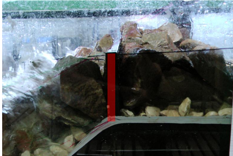
Figure 5. “Closed” – impermeable crest.
